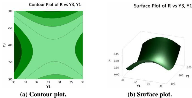
**Fig. 6. RSM plots for treadwear at speed = 40 kmph.**
