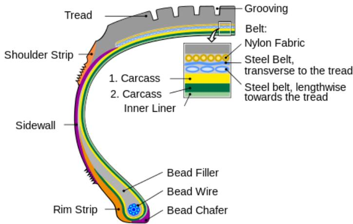
**Fig. 1. Components of a tire.**
