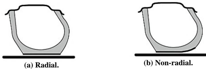
**Fig. 2. Ground sticking behaviour of tires.**
