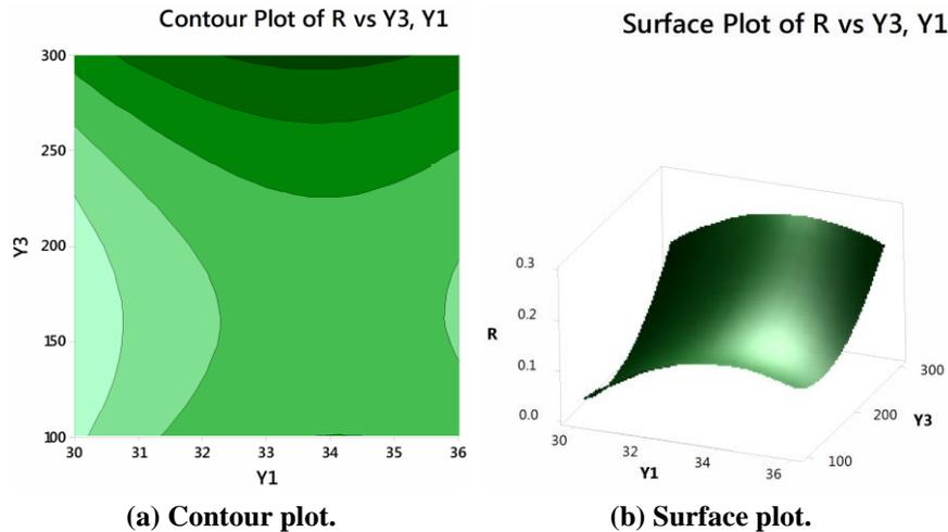
Fig. 7. RSM plots for treadwear at speed = 60 kmph.
