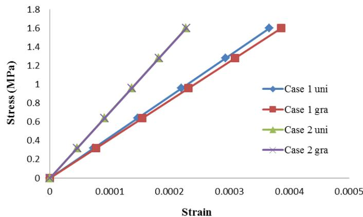
**Fig. 11 Stress-strain graph (elastic region) of case 1 and case 2 lattice structures**
