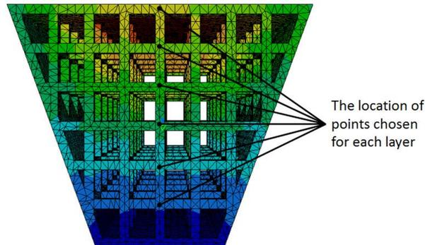
**Fig. 8. The points are chosen to compare the displacement value for uniform and lattice structure.**
