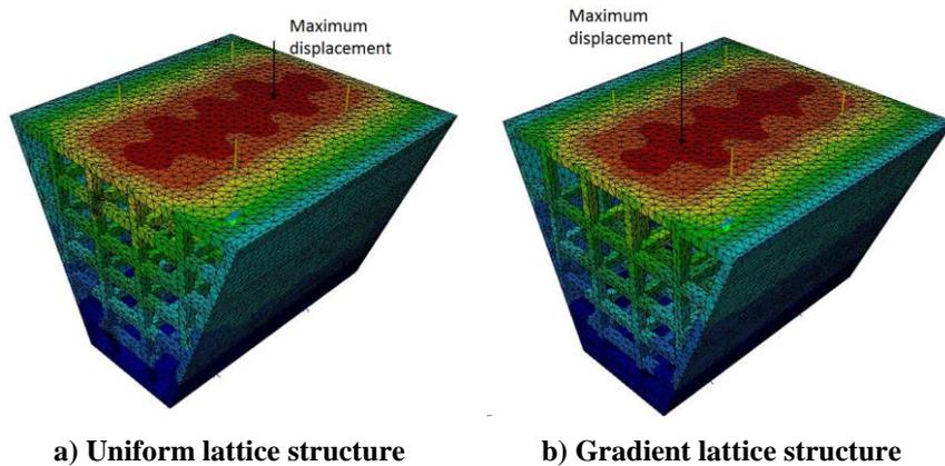
Fig. 9. FEA displacement analysis result for case 1.
