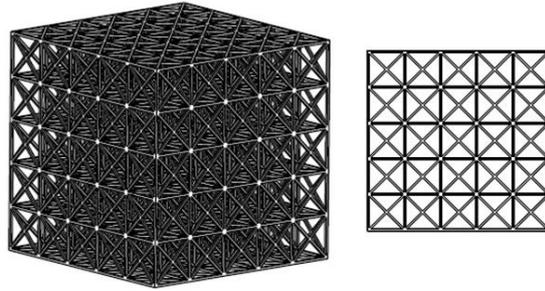
**Fig. 1. Isometric view and front view of the lattice structure.**
