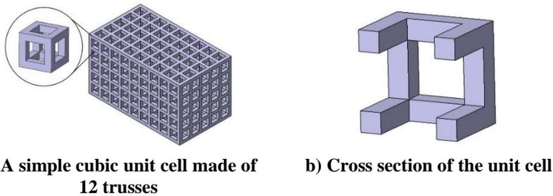
**Fig. 3. Simple cubic unit cells forming a uniform lattice structure.**
