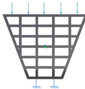
**Fig. 6. Load and clamping position for uniaxial compression test.**
