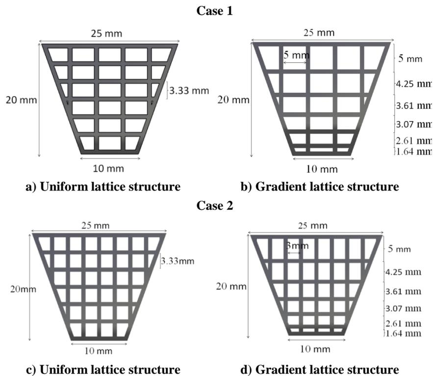
**Fig. 5. Dimensions of a) uniform and b) gradient lattice structure in case 1 and c) uniform and d) gradient lattice structure in case 2.**
