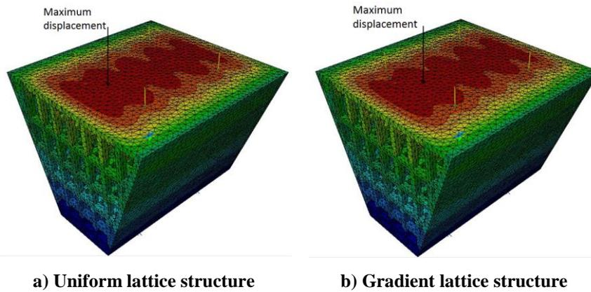
Fig. 9. FEA displacement analysis result for case 2.
