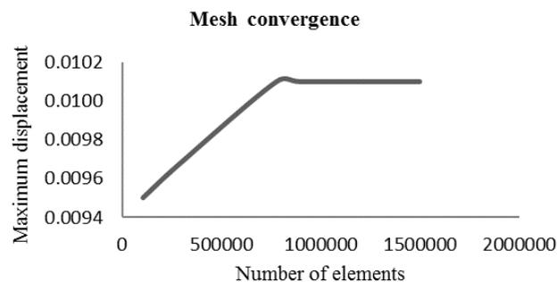
**Fig. 7. Mesh convergence test of maximum displacement value with the number of elements.**
