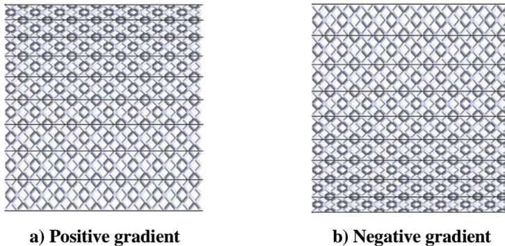
**Fig. 2. Step-wise rhombic dodecahedron gradient lattice structure with two types of progressivity a) positive gradient and b) negative gradient [13].**
