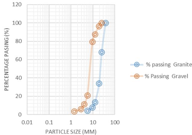
Fig. 3. Grading curves for granite and gravel.
