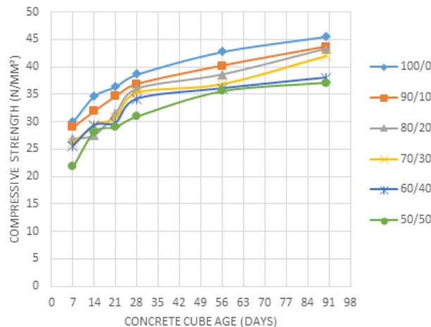
**Fig. 4. Interaction between compressive strength of SCC of varying granite/washed gravel and periods of immersion in days.**
