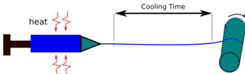
**Fig. 3. Pulling to a rotating drum.**
