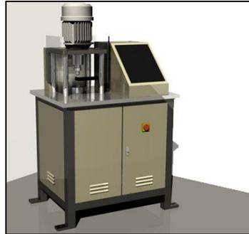
**Fig. 1. Photograph of a four-ball tester machine.**
