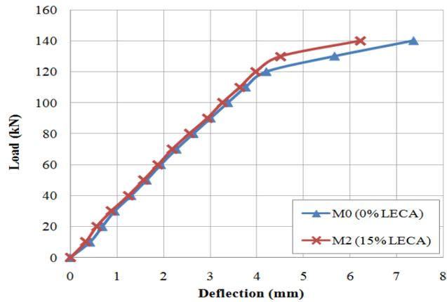
Fig. 12. Load vs average mid-span deflection of beams tested.
