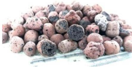
**Fig. 1. Light expanded clay aggregate (LECA).**
