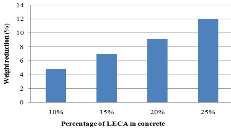
**Fig. 14. Weight reduction of concrete obtained corresponding to various percentage replacements of coarse aggregate with LECA.**
