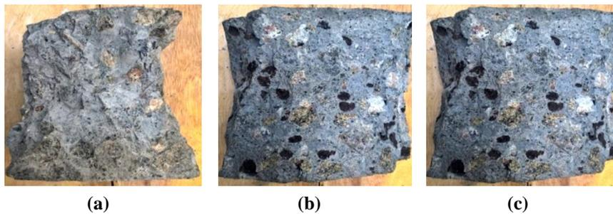
Fig. 9. Failure surface of concrete cubes: (a) M0 mix, (b) M2 mix, (c) M4 mix.
