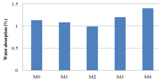
**Fig. 11. Water absorption results obtained for various concrete mixes.**
