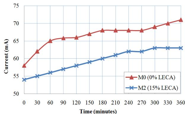
**Fig. 10. Current passed through concrete at various time intervals.**
