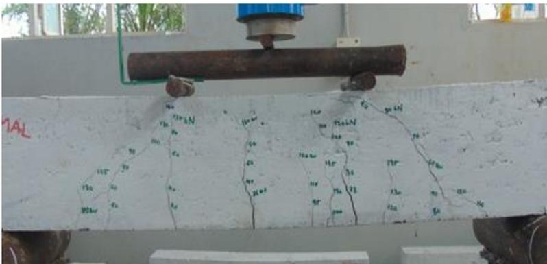
Fig. 13. Crack pattern of beam tested.
