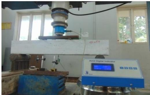
**Fig. 6. Experimental setup for determining flexural behaviour of RCC beams.**
