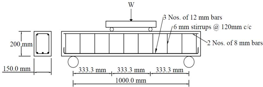
**Fig. 5. Reinforcement details of beam.**
