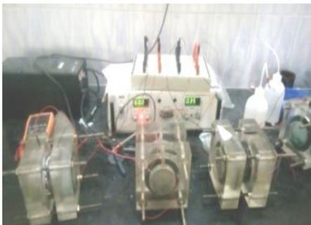
**Fig. 3. Rapid chloride penetration test.**
