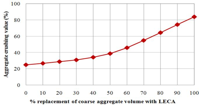
Fig. 7. Aggregate crushing value test results.
