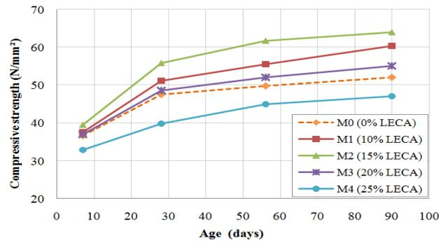
Fig. 8. Compressive strength of mixes measured at different ages of concrete.
