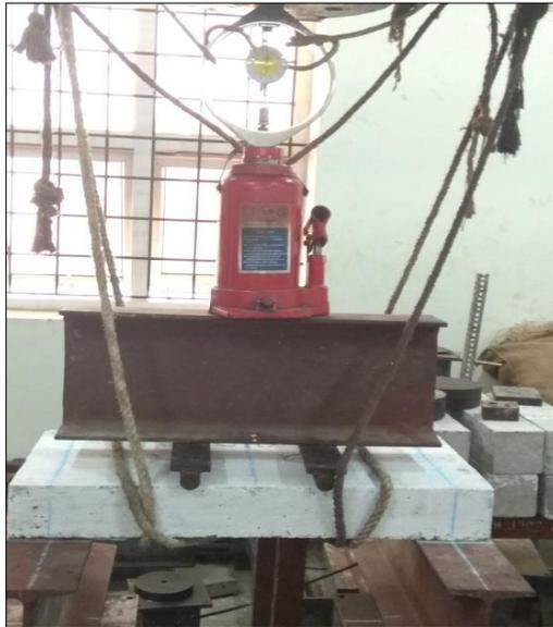
**Fig. 3. Slab panel subjected to flexural strength test.**
