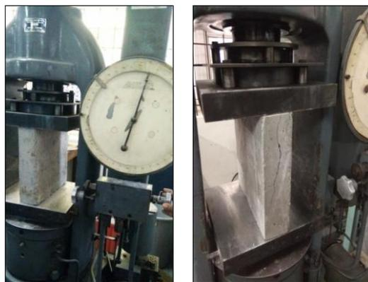
**Fig. 6. Wall panel under compression test.**
