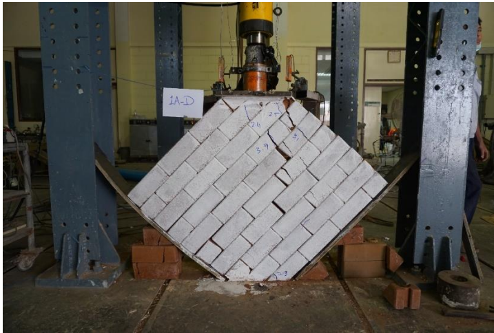
Fig. 8. Failure mode of the wall specimen W1.
