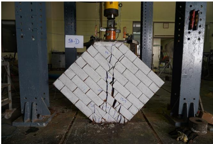
Fig. 12. Failure mode of the wall specimen W5-N-R.
