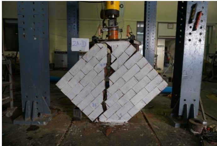
Fig. 9. Failure mode of the wall specimen W2-O.
