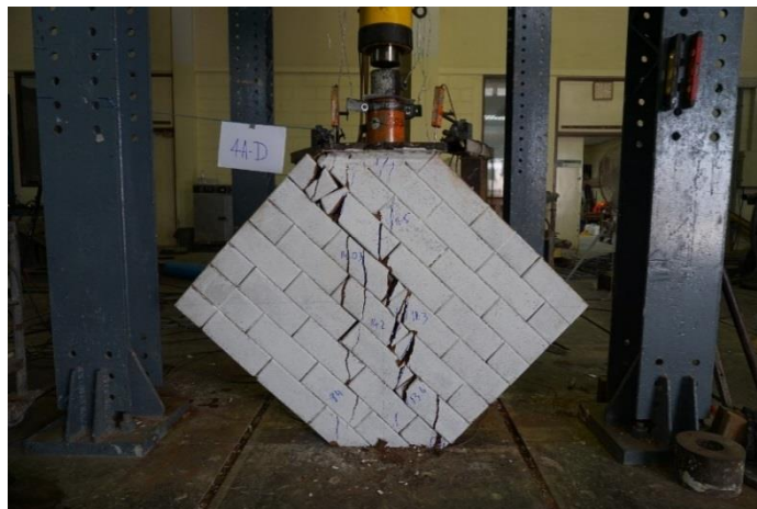
Fig. 11. Failure mode of the wall specimen W4-O-R.
