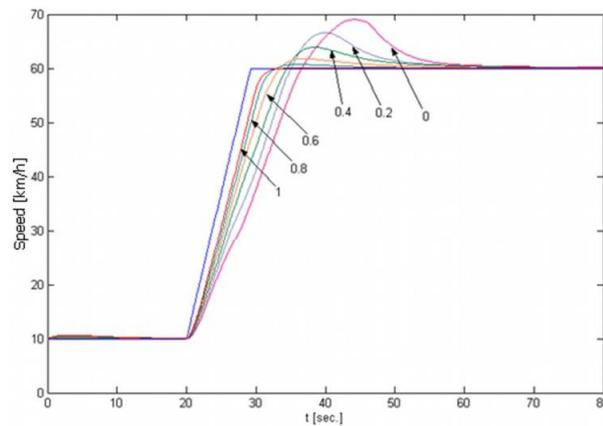
**Fig. 5. Output of simplified fuzzy model for different driving styles.**
