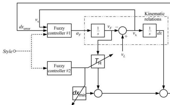
**Fig. 4. Structure of system for trajectory generation, based on simplified fuzzy controller.**
