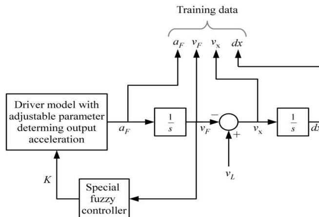
Fig. 9. Block diagram of model for generating training data.
