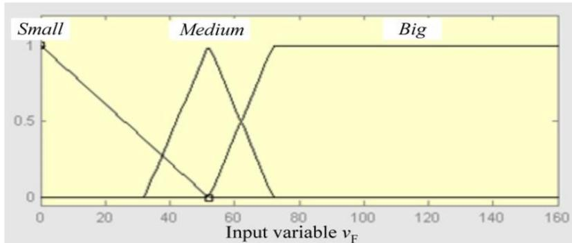
**Fig. 10. Membership functions of the input variable  $v_f$  of special fuzzy controller.**
