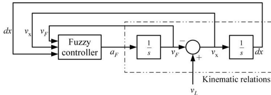
**Fig. 3. Block structure of driver model based on fuzzy controller with three inputs.**
