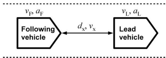
Fig. 1. Parameters in longitudinal motion.
