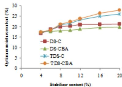
Fig. 5. Variation of OMC at different stabilizer content.
