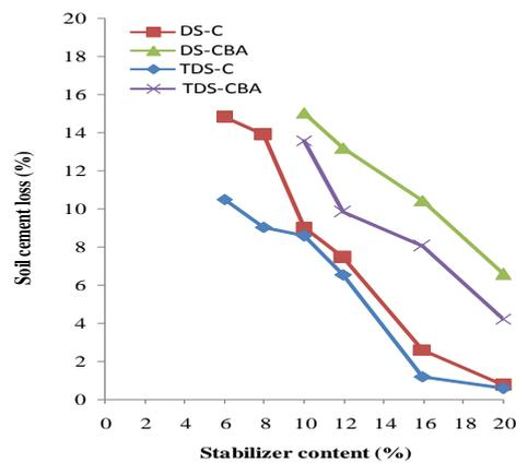
Fig. 8. Variation of percentage soil-cement losses.
