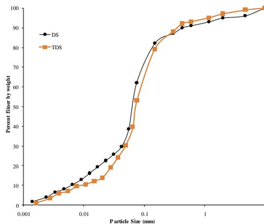
Fig. 3. Particle size distribution curve of DS and TDS.
