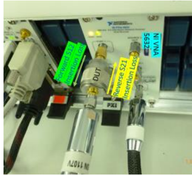
Fig. 6. A DUT measured S12 and S21 in network analyser.
