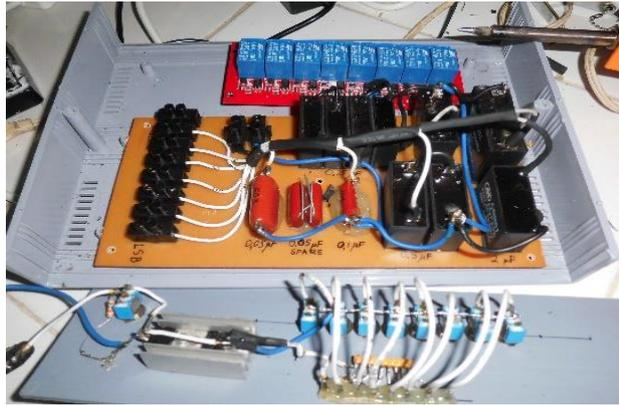
Fig. 3. Binary combination switches and excitation capacitors.
