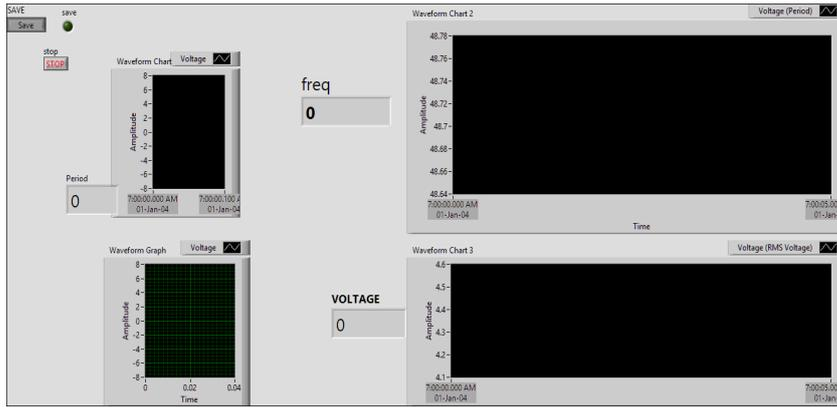
**Fig. 9. Labview VI front panel of voltage and frequency data acquisition.**
