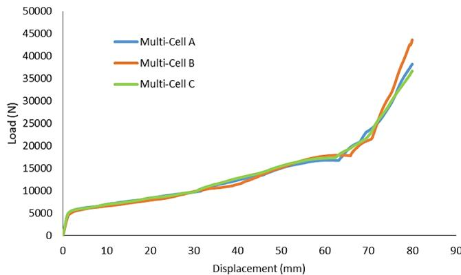
**Fig. 7. Load-displacement curve of multi-cell thin-walled circular tubes.**
