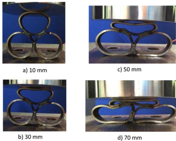
**Fig. 11. Deformation mode of a multi-cell thin-walled circular tube under quasi-static lateral loading.**
