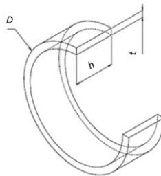
Fig. 2. Schematic diagram of thin-walled circular tube.
