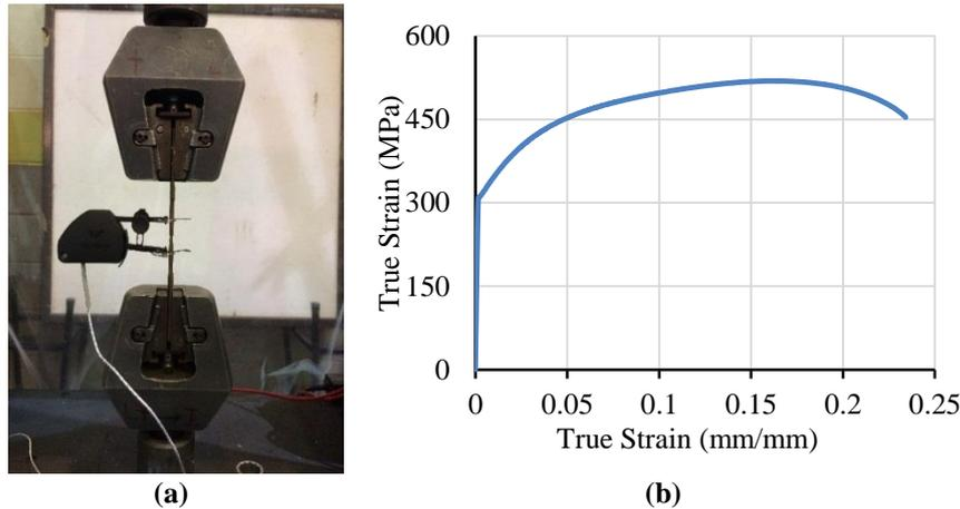
Fig. 1(a) Tensile test set-up by using INSTRON 5982,
