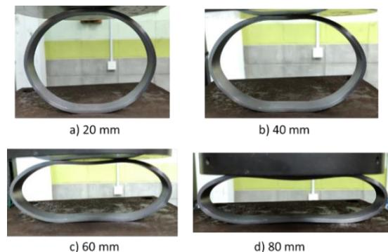
Fig. 10. Deformation mode of large single thin-walled circular tube under quasi-static lateral loading.
