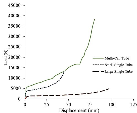
Fig. 8. Load-displacement curve of each thin-walled circular tubes.
