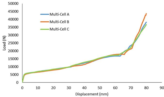
**Fig. 7. Load-displacement curve of multi-cell thin-walled circular tubes.**
