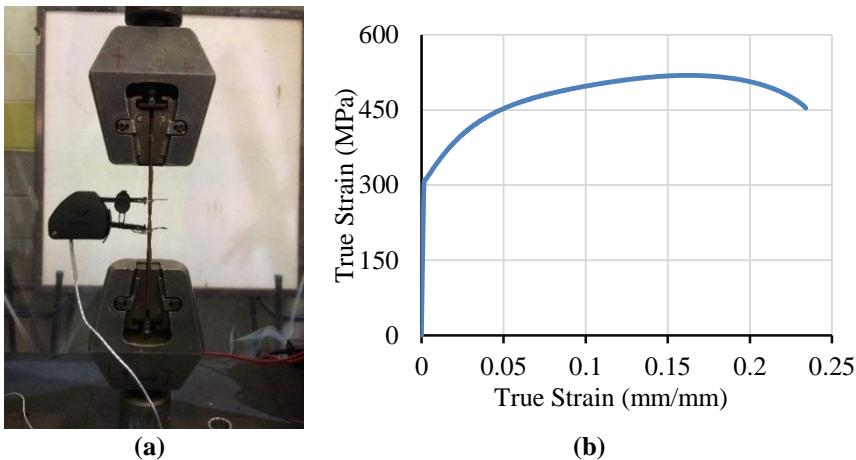
**Fig. 1(a) Tensile test set-up by using INSTRON 5982,
