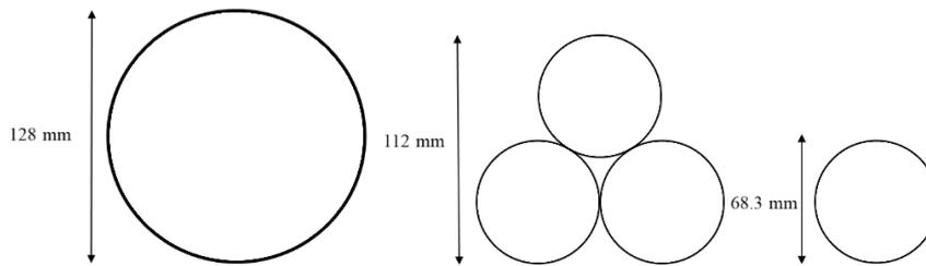
**Fig. 3. Schematic diagram of thin-walled circular tube configuration.**
