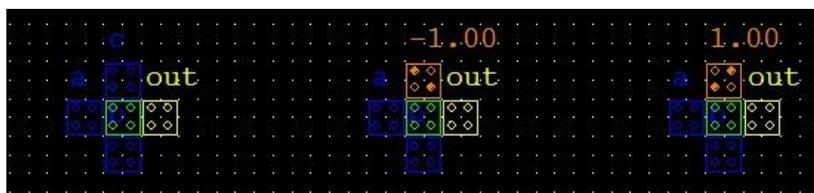
Fig. 2. Majority gate with polarization phenomenon [10].
