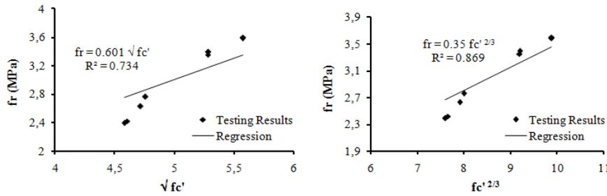
**Fig. 7. Relationships between modulus of rupture and compressive strength for pumice lightweight concrete.**
