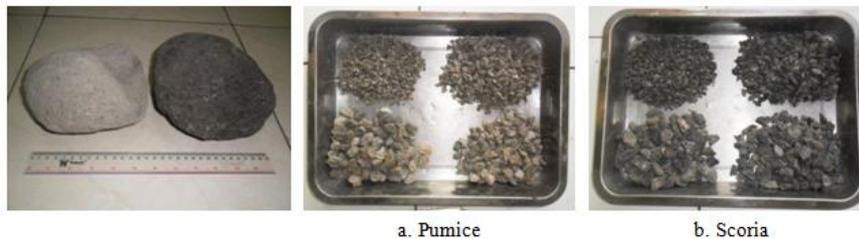
**Fig. 1. Pumice, scoria and four different particle sizes of coarse aggregates.**
