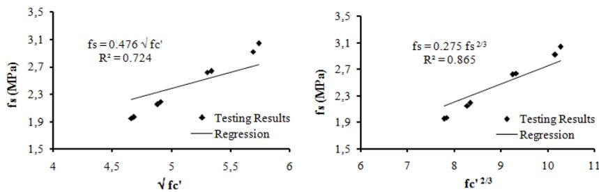
**Fig. 6. Relationships between splitting tensile and compressive strength for scoria lightweight concrete.**
