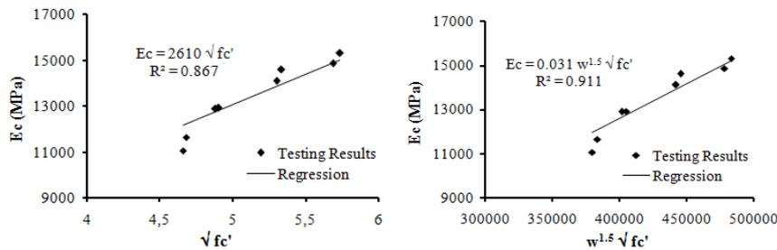
**Fig. 4. Relationships between modulus of elasticity and compressive strength for scoria lightweight concrete.**
