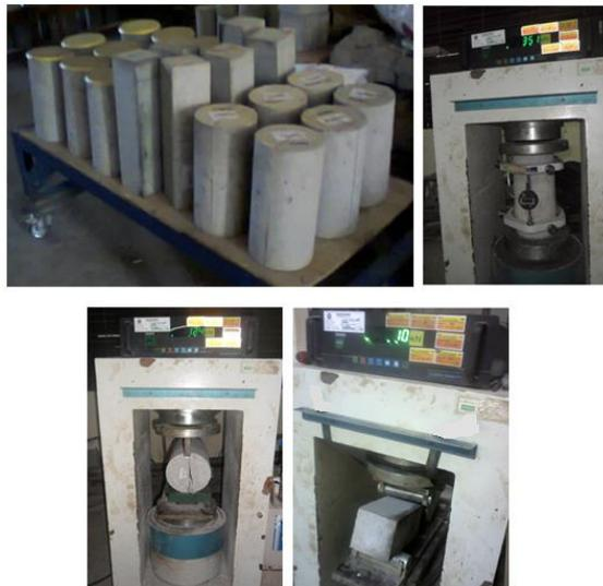
**Fig. 2. Specimens and mechanical properties tests.**
