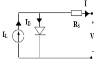
(b) Simplified equivalent circuit with  $R_s$
