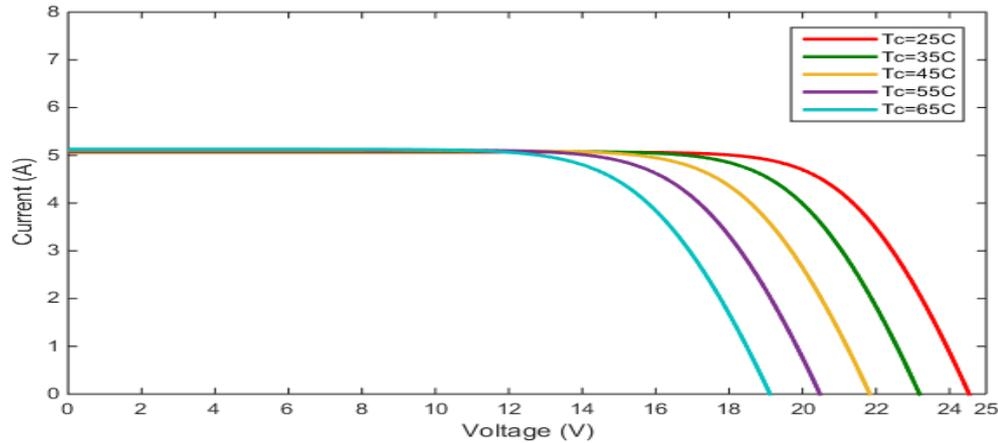
**Fig. 17. I-V characteristic of the PV module at various cell temperature and constant solar radiation.**
