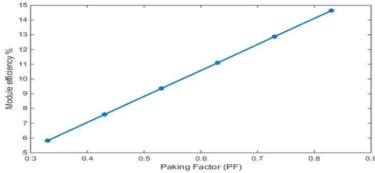
**Fig. 11. Effect packing factor on module efficiency.**
