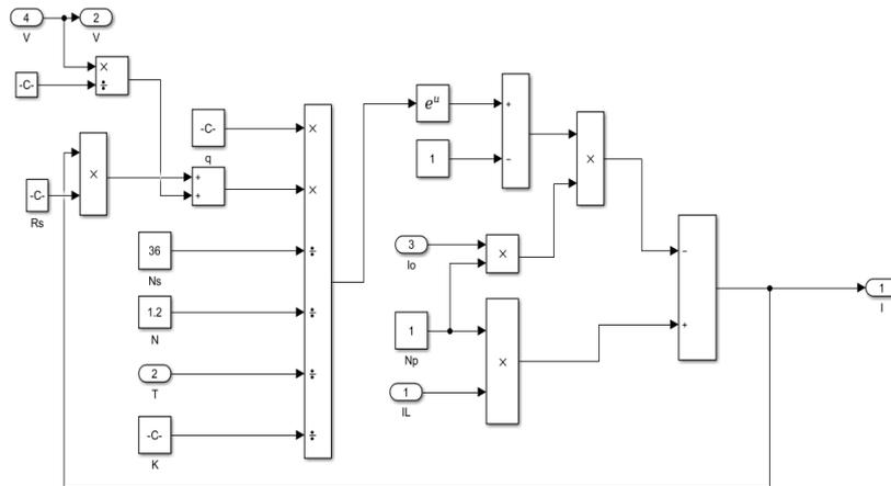
**Fig. 9. Output current of PV module.**
