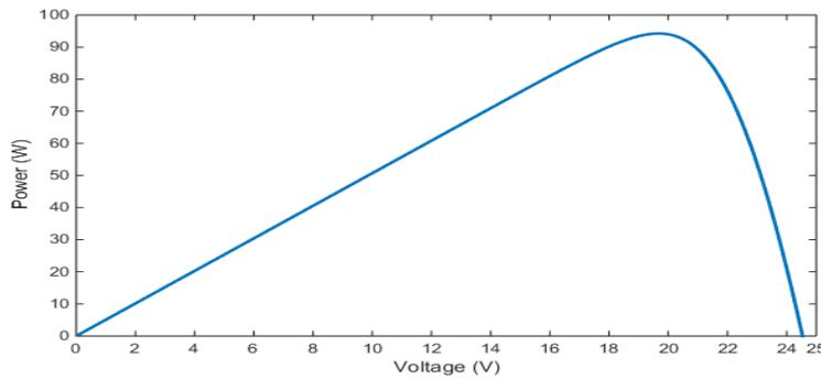
**Fig. 12. P-V characteristic of the proposed PV module at STC.**
