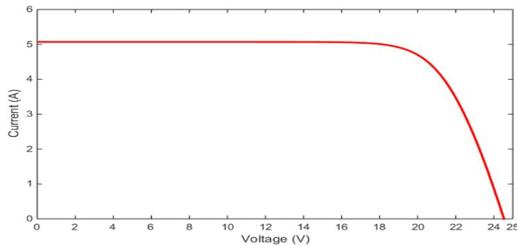
**Fig. 13. I-V characteristic of the proposed PV module at STC.**
