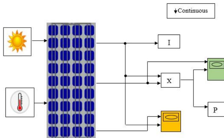
**Fig. 10. Block diagram of simulink model.**
