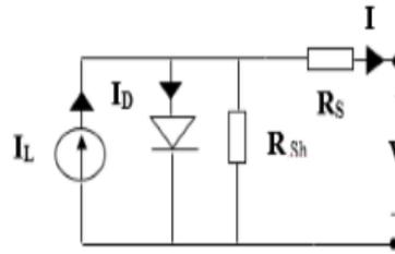
(a) Equivalent circuit with  $R_{sh}$  and  $R_s$
