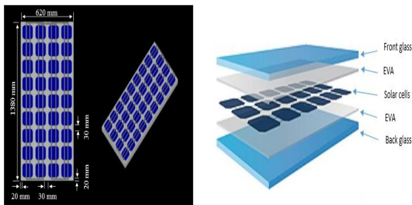
(a) Layout of the designed PV module.
