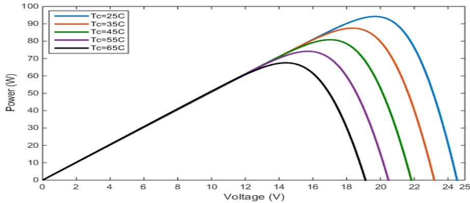
**Fig. 16. P-V characteristic of the PV module at various cell temperature and constant solar radiation.**
