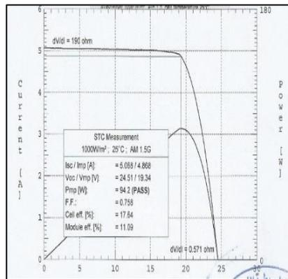
(f) Tested result of PV module.
