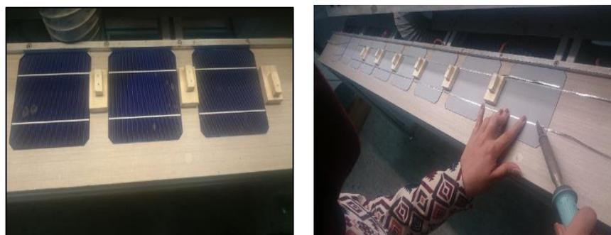
(a) Wooden structure between cells.
