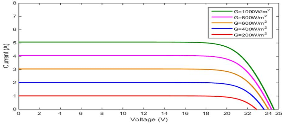
**Fig. 14. I-V characteristic of the PV module at various solar radiation and constant cell temperature.**
