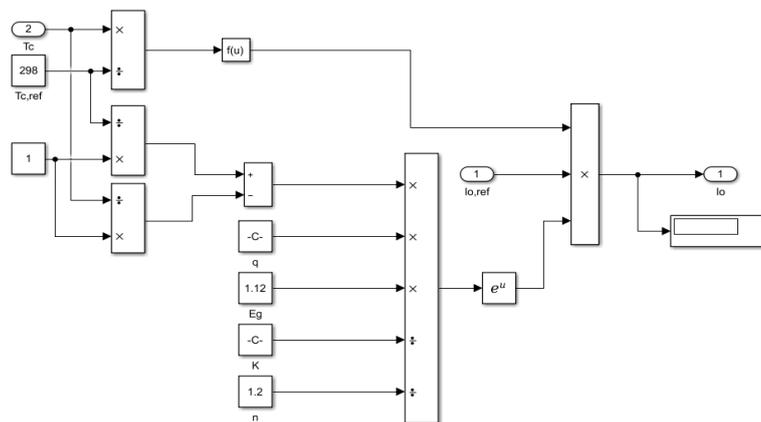
Fig. 8. Model of saturation current of diode.
