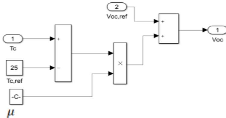
Fig. 7. Model of open circuit voltage.
