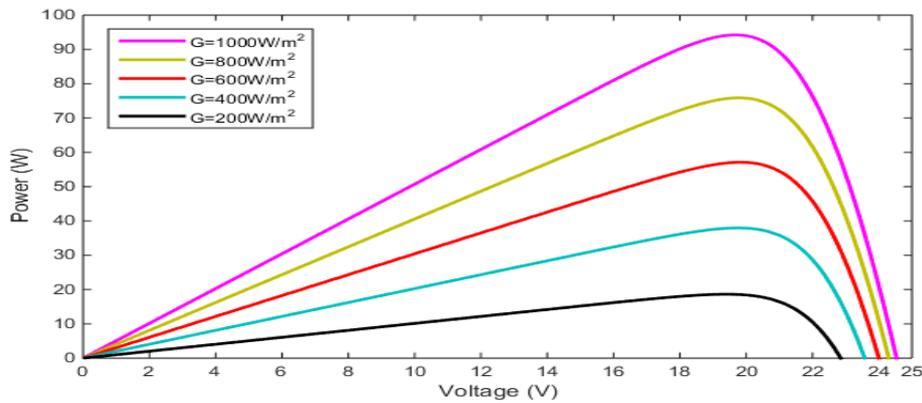
**Fig. 15. P-V characteristic of the PV module at various solar radiation and constant cell temperature.**
