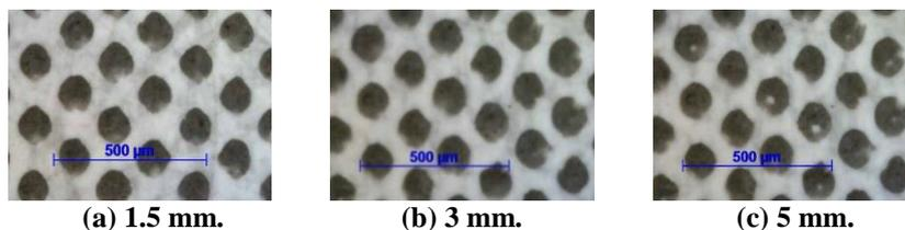
Fig. 7. Dot structures on 50 GSM.
