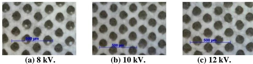
Fig. 6. Dot structures on 65 GSM.
