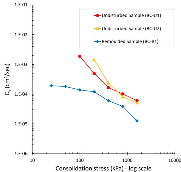
**Fig. 4. Variation of  $C_v$  with consolidation stress for an undisturbed and remoulded sample.**
