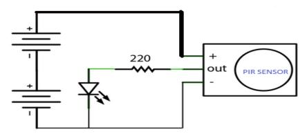
Fig. 6. Circuit for testing PIR sensor.
