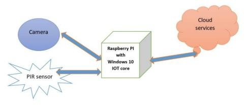
Fig. 5. Architecture of intrusion detection system.
