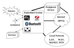
Fig. 1. Typical architecture of Internet of Things (IoT).
