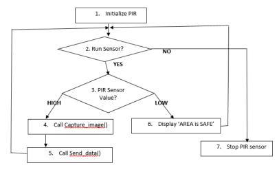
Fig. 7. Control flow graph (CFG) for the intrusion system.
