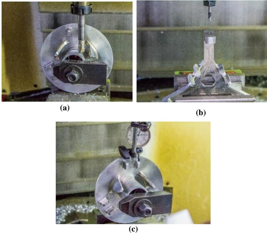
**Fig. 11. The various machining processes involved in fabrication of the CVT. (a) shows roughing cycle, (b) shows the drilling cycle and (c) shows the verification of tolerances using a dial gauge.**
