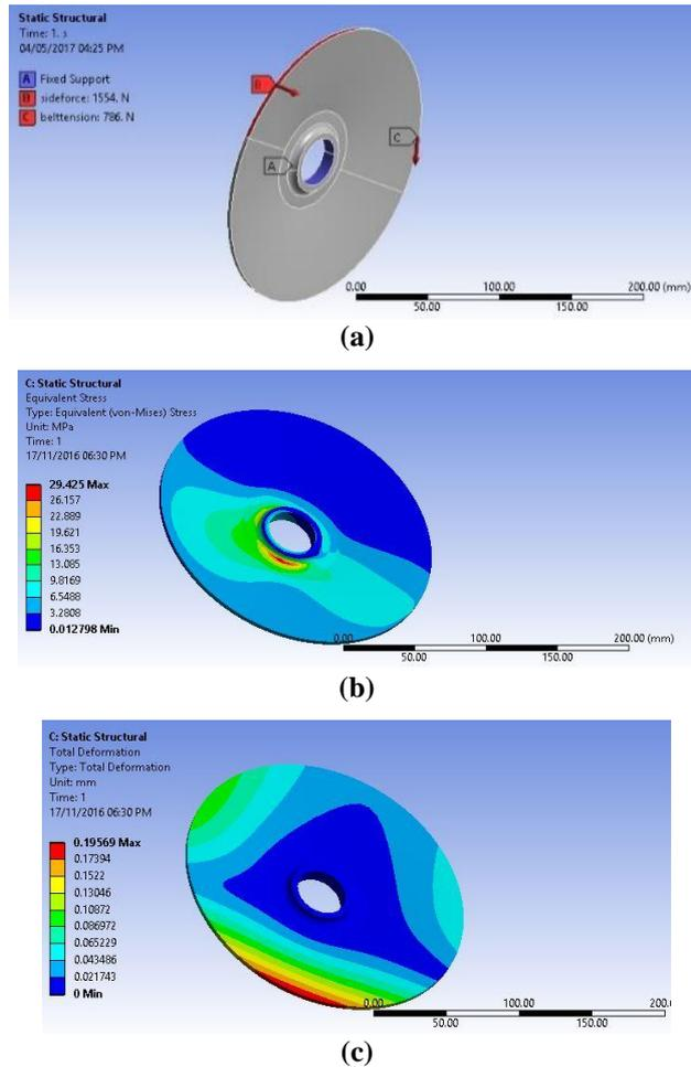
**Fig. 10. The loading condition (a), stress concentration (b) and deformation (c) of the driven pulley fixed sheave.**
