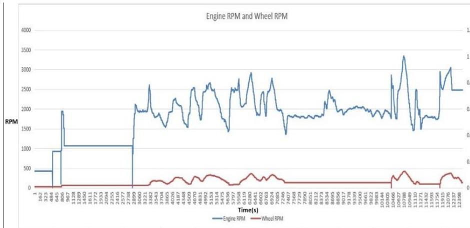
Fig. 1. The plot of wheel RPM and engine RPM vs. time in seconds.
