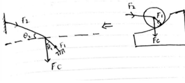
Fig. 3. Freebody diagram of the pulley.
