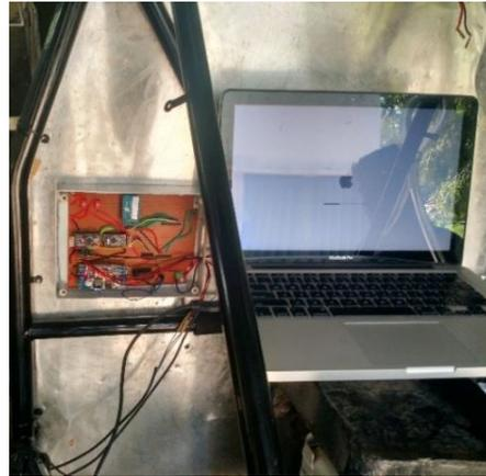
**Fig. 12. The DAQ system installed on the ATV.**
