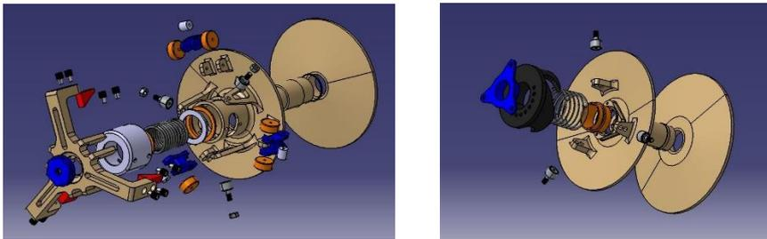
Fig. 5. (a) and (b) depicts the exploded view of the drive and driven pulley of the designed continuously variable transmission respectively.
