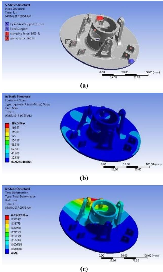
**Fig. 6. The loading condition (a), stress concentration (b) and deformation (c) of the drive pulley moveable sheave.**
