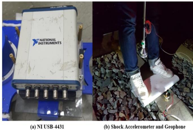
Fig. 7. Data acquisition device and sensors used during the field test.
