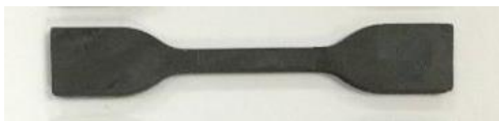
Fig. 1. Dumbbell test piece.
