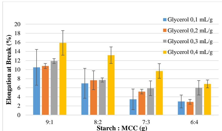
**Fig. 3. The effect of MCC from sugar palm fiber and glycerol addition on elongation at break of bioplastics.**
