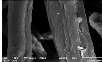
**Fig. 5(b). MCC from Sugar Palm Fiber Using a Magnification of 5000x.**
