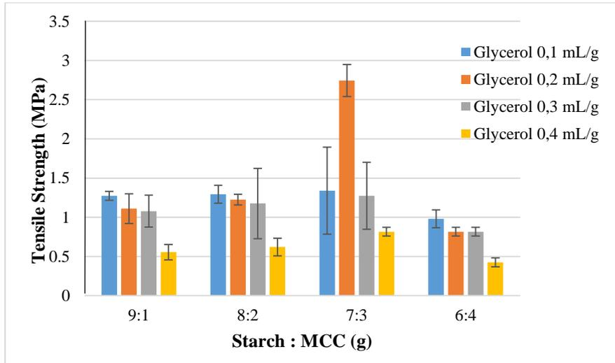
**Fig. 1. The effect of MCC from sugar palm fibers and glycerol addition on tensile strength of bioplastics.**
