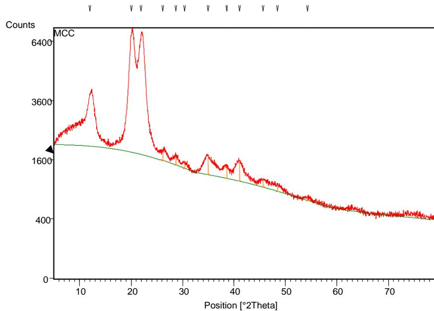
**Fig. 1. XRD patterns of MCC samples derived from sugar palm fibers.**
