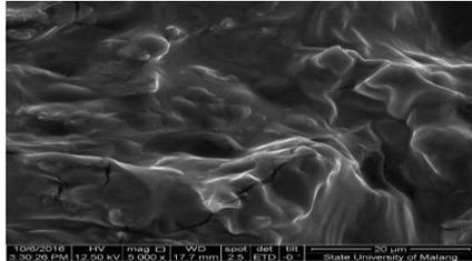
**Fig. 5(a). Fractures Bioplastics with Filler MCC and Plasticizer Glycerol Using a Magnification of 5000x.**
