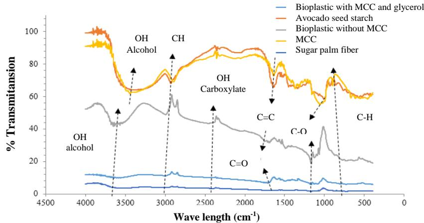
**Fig. 4. The FTIR analysis results of avocado seeds starch, MCC, sugar palm fiber, bioplastic from avocado seeds starch without MCC, and bioplastic from avocado seeds starch with MCC and glycerol.**
