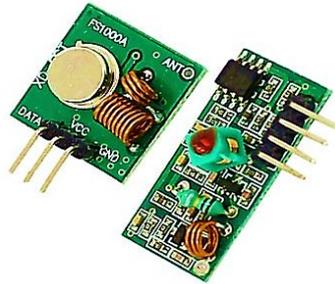
Fig. 2. RF wireless module used in this research, left transmitter, right receiver.
