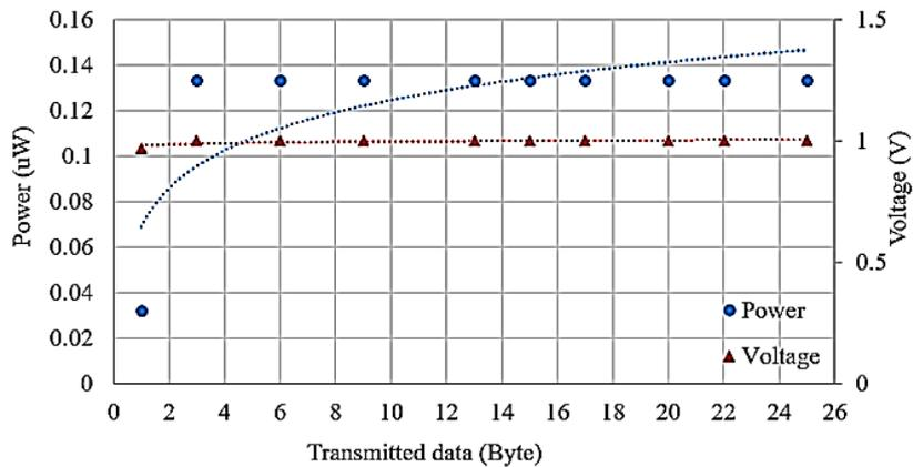
**Fig. 7. Minimum power and voltage drawn by the conventional RF transmitter circuit during the sleep mode.**
