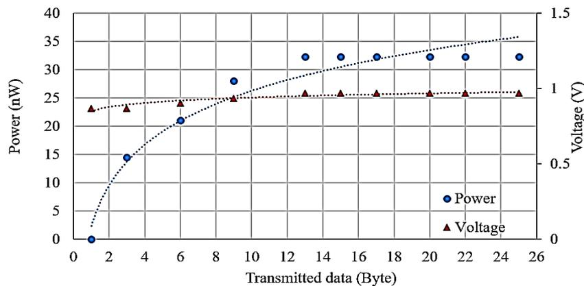
**Fig. 10. Minimum power and voltage drawn by the proposed enhanced RF transmitter circuit during the sleep mode.**
