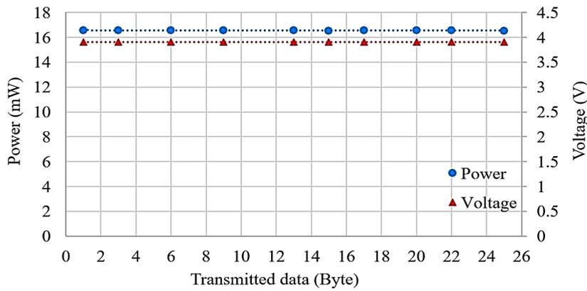
**Fig. 13. Minimum power and voltage drawn by the RF receiver module.**
