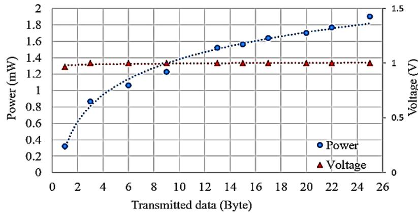
**Fig. 6. Minimum power and voltage drawn by the conventional RF transmitter circuit during the active mode.**
