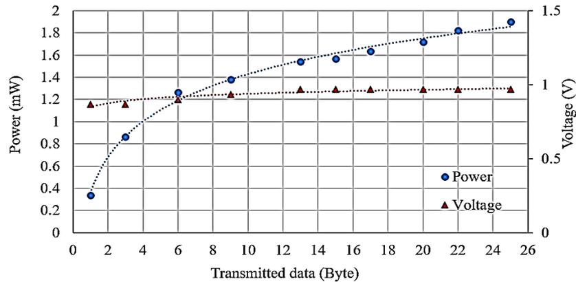
**Fig. 9. Minimum power and voltage drawn by the proposed enhanced RF transmitter circuit during the active mode.**
