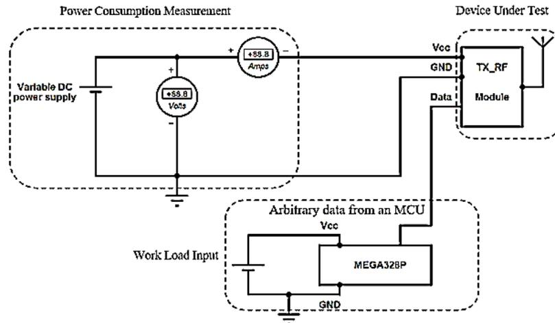
Fig. 5. Characterization of the conventional RF transmitter circuit.
