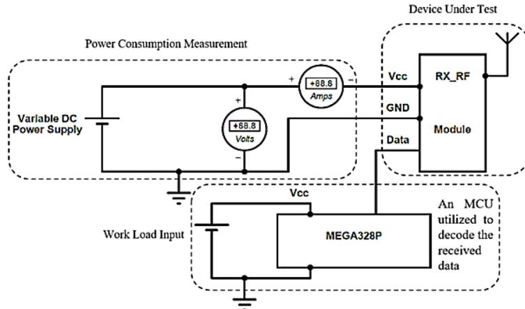
**Fig. 12. Characterization circuit for RF Receiver.**
