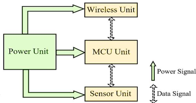
**Fig. 1. Typical wireless sensor node block diagram.**
