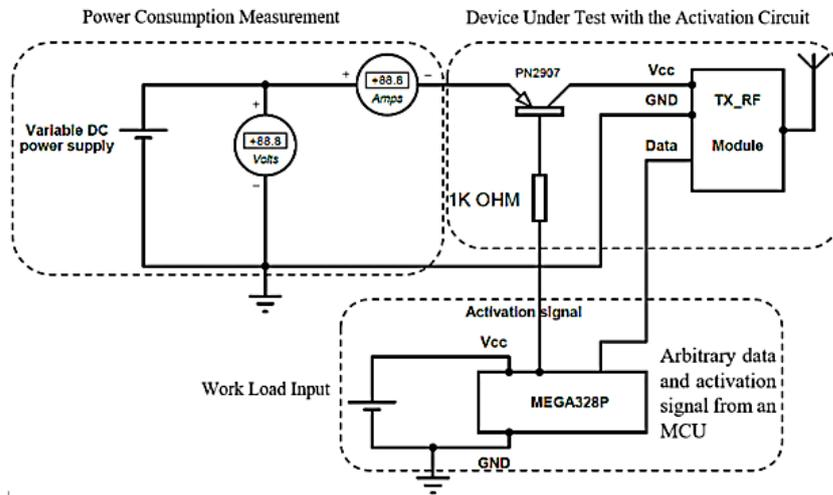
**Fig. 8. Characterization of the proposed enhanced RF transmitter circuit.**
