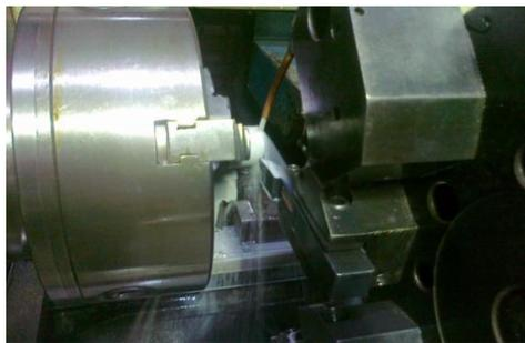
(a) CNC machine in wet condition.
