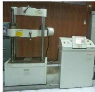
(b) Universal testing machine used for tensile test of steel bar.
