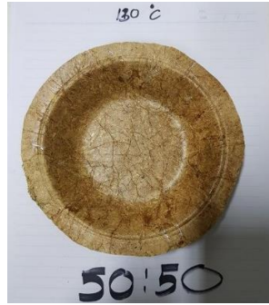
Fig. 6. Shows forming of water hyacinth ware.
