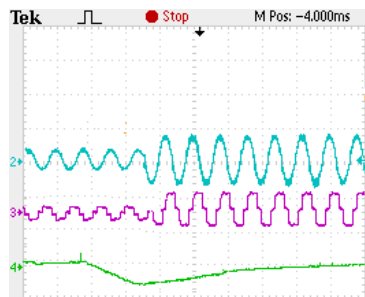
(a) Step load increase, source current (CH2: Y-axis: 3A/div, X-axis: 25ms), load current (CH3- Y-axis: 3A/div, X-axis: 25ms), DC-link voltage (CH4: Y-axis-150V/div).
