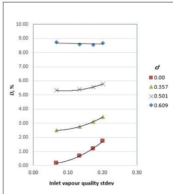
**Fig. 9. Trend of  $D$  vs. inlet vapour quality standard deviation (Mean inlet quality = 0.65, skew = 0.00) for the case of uniform and non-uniform (Normalized standard deviation = 0.357, 0.501, 0.609 and skew = 0.00) flow distribution.**
