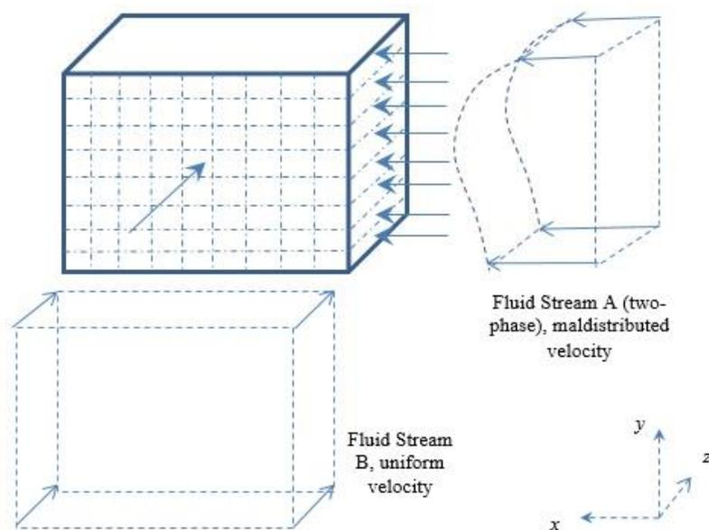
**Fig. 1. Representation of cross-flow heat exchanger with maldistributed two-phase flow.**
