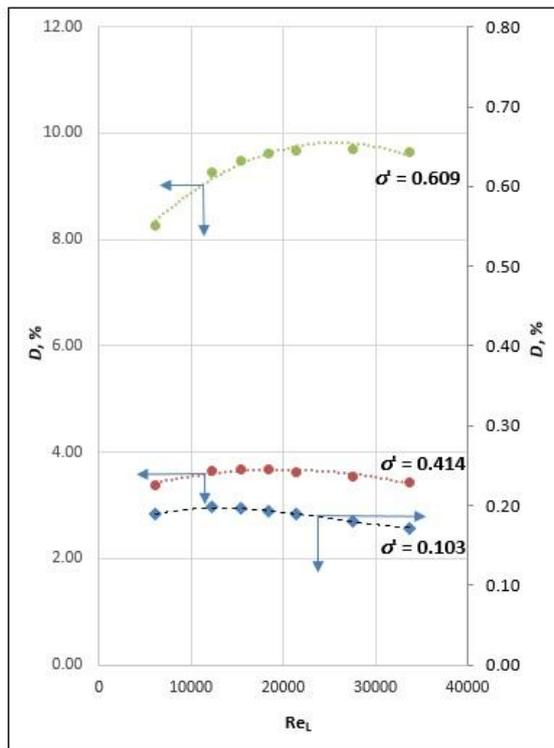
Fig. 7. Trends of  $D$  vs. liquid Reynolds number at specific flow distribution normalized standard deviation (Skew = 0.00).
