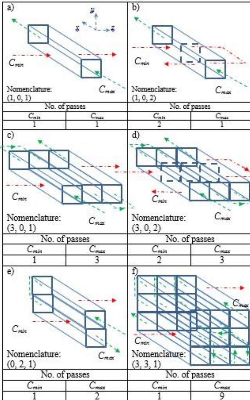
Fig. 2. Examples of pass configurations through heat exchanger.
