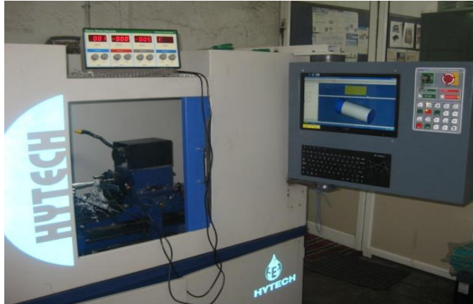
Fig. 2. CNC lathe fixed with strain gauge dynamometer.
