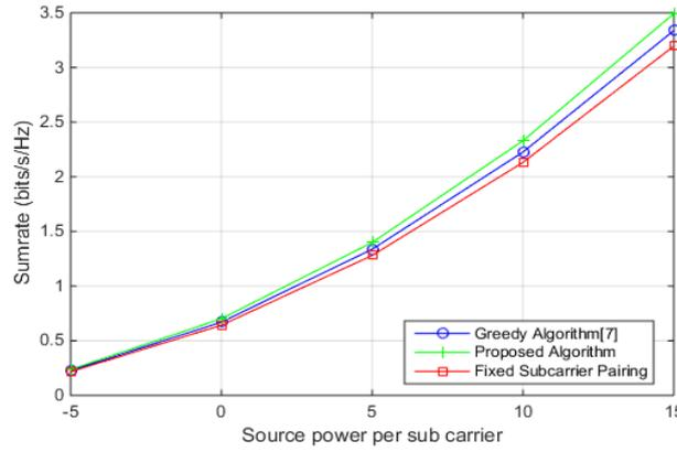
Fig. 4. Performance comparison of the proposed Prim's algorithm with Greedy algorithm [7] and benchmark.
