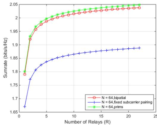
Fig. 5. Effects of the number of relays, where  $N = 64, K = 5,$  and  $P_{kl} = 10$  dB.
