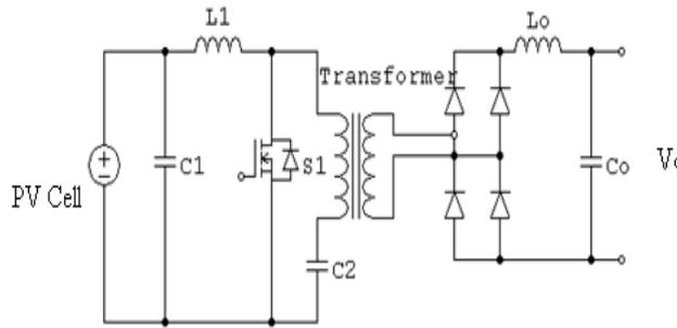
**Fig. 14. Single switch isolated DC-DC converter.**
