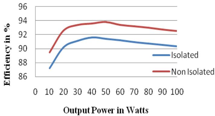
Fig. 22. Efficiency comparison -isolated and non-isolated converters.
