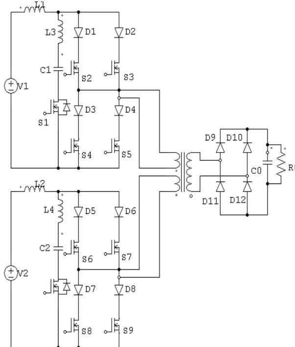
**Fig. 13. Two-Input current fed full bridge DC-DC converter.**
