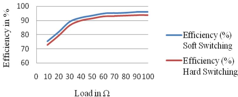
Fig. 9. Efficiency comparisons - HSBC and SSBC.
