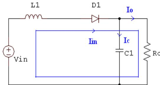
**Fig. 4. Boost converter - MOSFET OFF.**
