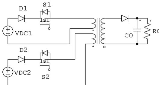
Fig. 12. Basic two-input DC-DC converter.
