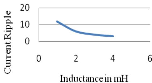
**Fig. 5. Inductor vs. current ripple.**
