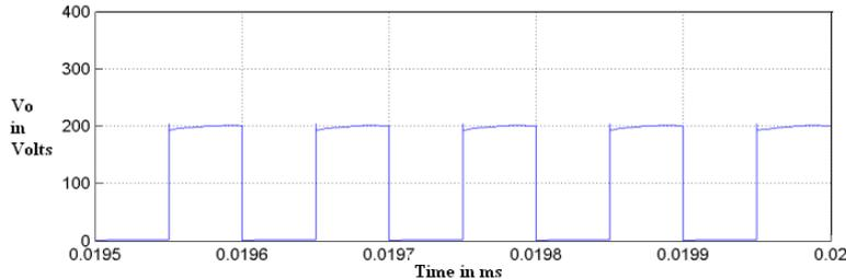
**Fig. 7. Output DC voltage of boost converter.**
