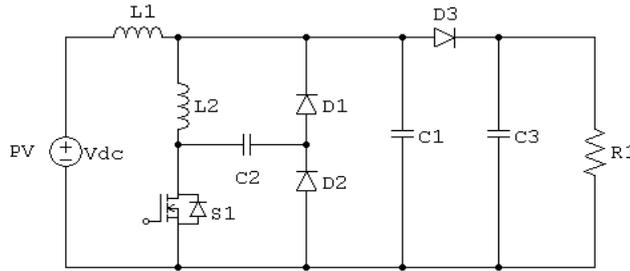
**Fig. 8. Single switch soft switching boost converter.**
