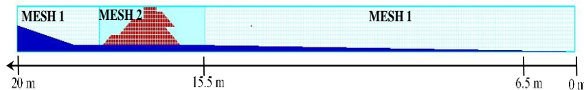
Fig. 2. Computational boundary meshing for numerical wave flume.
