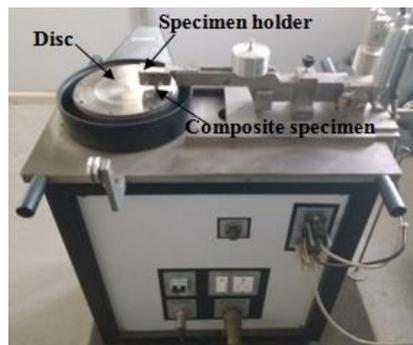
**Fig. 1. Pin-on-disc tribometer.**
