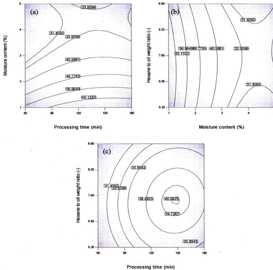
**Fig. 3. Contour plots showing the effects of experimental factors on biodiesel yield: (a) processing time and moisture content at hexane to oil weight ratio of 7.6, (b) moisture content and hexane to oil weight ratio at processing time of 120 min, and (c) processing time and hexane to oil weight ratio at moisture content of 3%.**
