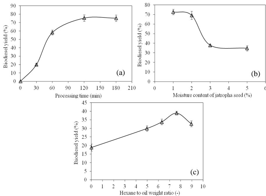
**Fig. 2. Effect of process parameters on yield of biodiesel**
