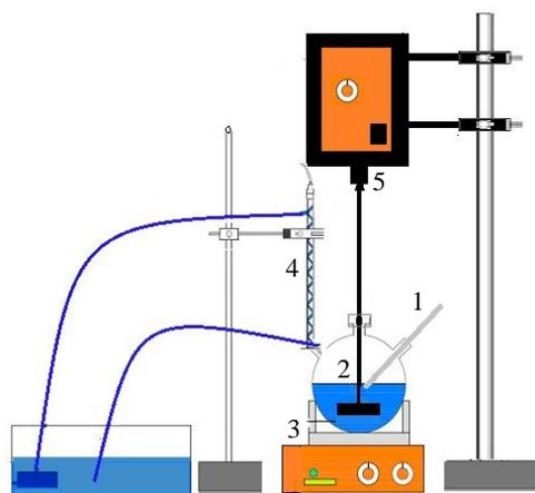
**Fig. 1. Schematic apparatus for reactive-extraction of jatropha seed: 1 - thermometer, 2 - reaction mixture, 3 - water bath, 4 – condenser, 5 - agitation motor**
