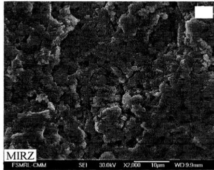
Fig. 6. MIRZ section where lamellar structure is damaged [23].
