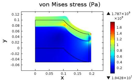
**Fig. 12. Von Mises stress after transformation.**
