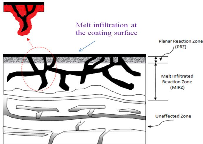
**Fig. 1. Typical coating section showing planar reaction and melt infiltrated reaction zones.**
