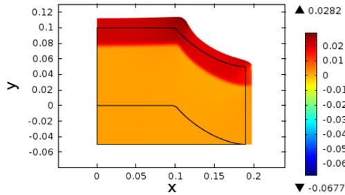
**Fig. 11. Volumetric (swelling) strain after transformation.**
