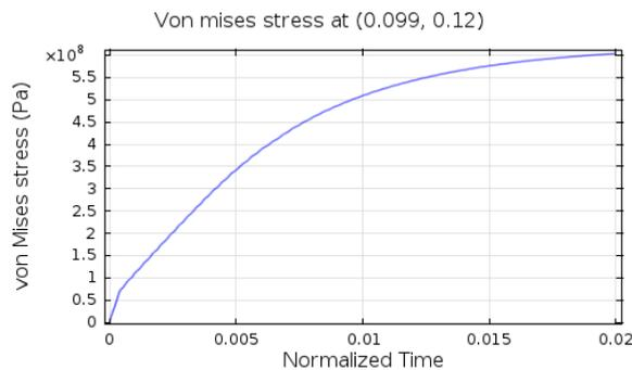
**Fig. 15. Variation of Von Mises stress with time.**
