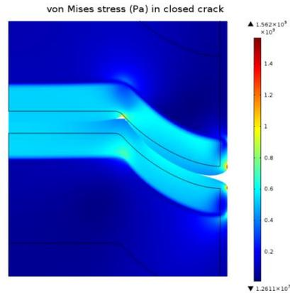
**Fig. 14. Von Mises stress after crack closure.**
