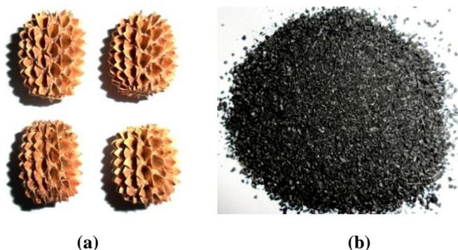
**Fig. 1. Photographs of (a) the dried APCs raw material and (b) the APCs activated carbon.**
