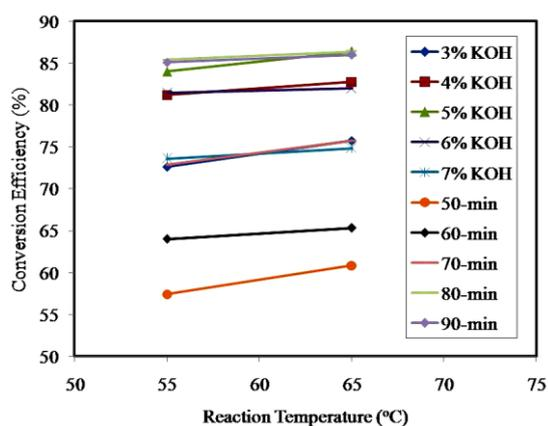
**Fig. 6. Effect of reaction temperature on the biodiesel production from the SPFS using in-situ transesterification with the assistance of ultrasound. Experimental conditions: 25:1 w/w ratio of methanol to the SPFS oil, 1:1 w/w ratio of methanol to chloroform, 3-7% KOH and 50 rpm stirring, 37 kHz ultrasound, 55-65 °C reaction temperature, 50-90-min reaction time. An average value of multiplied run was taken, and the standard deviation was 0.552 on average.**
