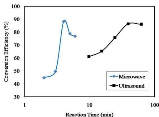
**Fig. 2. Effects of reaction time on the biodiesel production from the SPFS using in-situ transesterification. Experimental conditions: 25:1 w/w ratio of methanol to the SPFS oil, 1:1 w/w ratio of methanol to chloroform, 5% KOH and 50 rpm stirring (1) Ultrasound assistance: 37 kHz ultrasound, 65 °C reaction temperature (2) Microwave assistance: 450W, hold at 65 °C. An average value of multiplied run was taken, and the standard deviation was 0.635 on average.**
