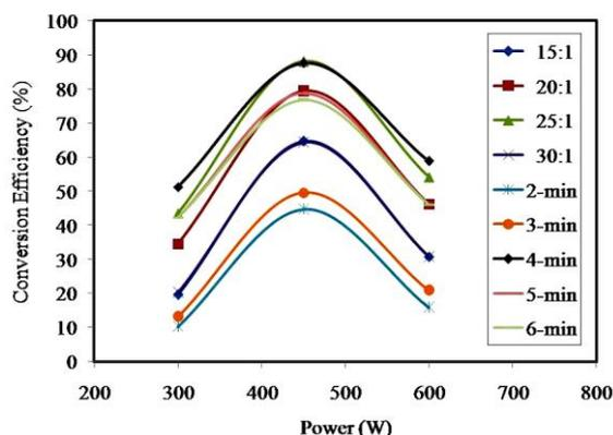
**Fig. 5. Effect of microwave power on the biodiesel production from the SPFS using in-situ transesterification. Experimental conditions: 15:1 to 30:1 w/w ratio of methanol to the SPFS oil, 1:1 w/w ratio of methanol to chloroform, 5% KOH, 50 rpm stirring, 300-600W, 2-6-min reaction time. An average value of multiplied run was taken, and the standard deviation was 0.481 on average.**
