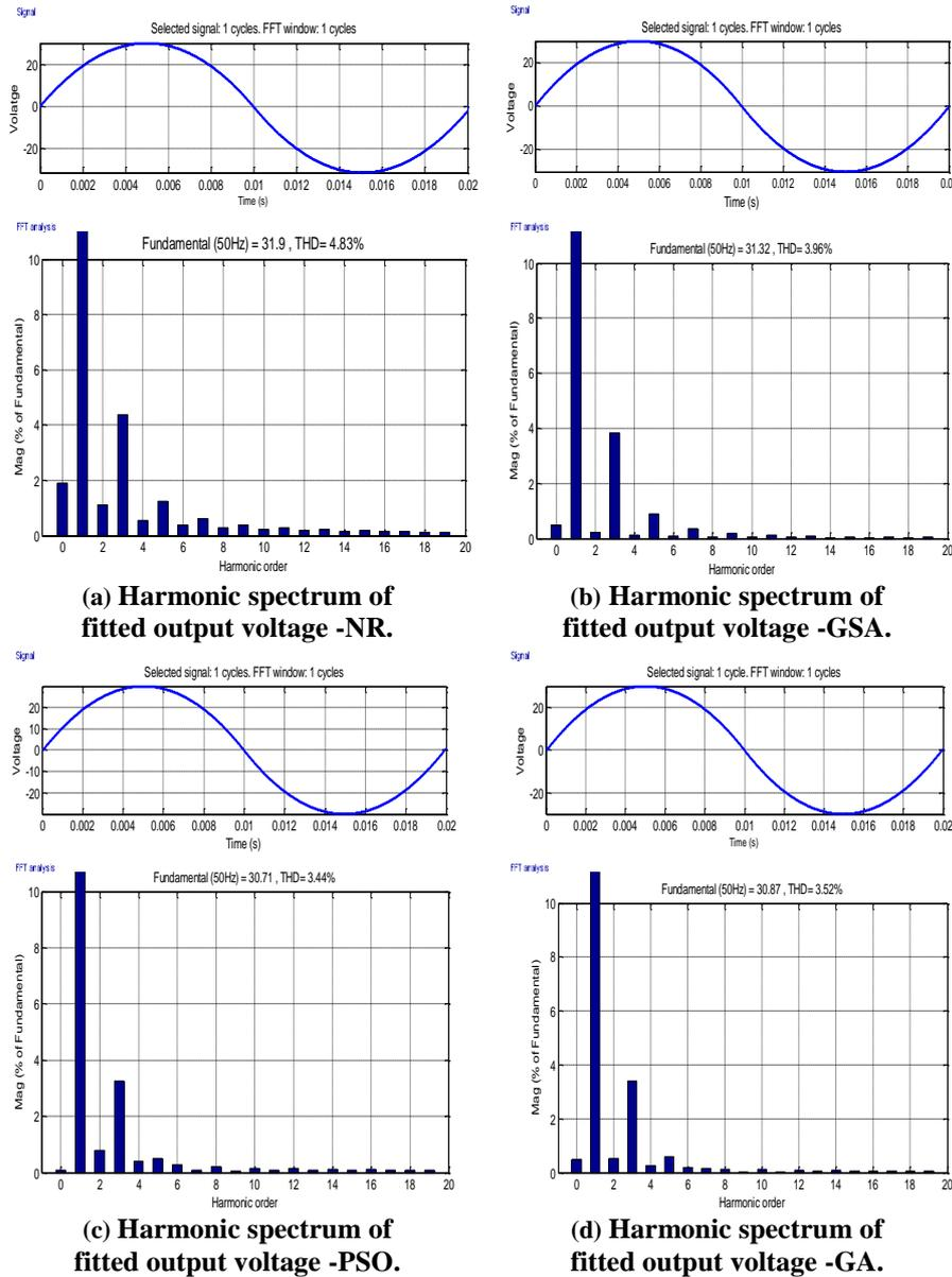
**Fig. 6 FFT results of SC techniques with curve fitting.**
