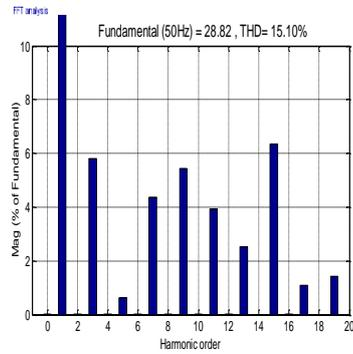
(d) FFT analysis of 7 level inverter output voltage using GA.
