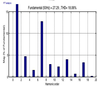
**(a) FFT analysis of 7 level Inverter output voltage using NR**
