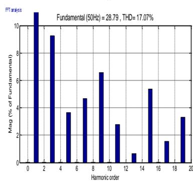
**(b) FFT analysis of 7 level Inverter output voltage using GSA.**
