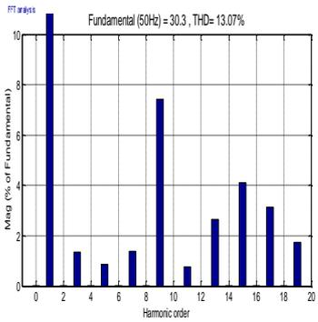
(c) FFT analysis of 7 level inverter output voltage using PSO.
