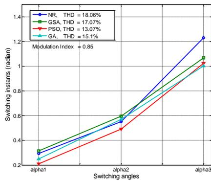
Fig. 5(a) switching instants for SC techniques.
