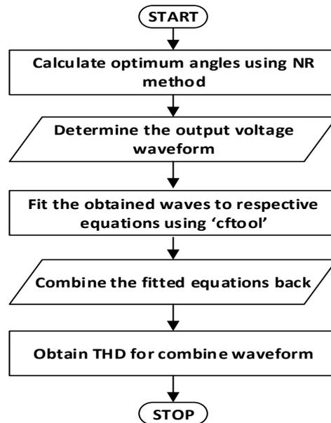
Fig. 2. Flowchart-NR based piecewise curve fitting.
