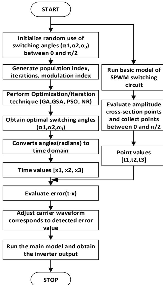
Fig. 1. Flow chart for PWM switching calculation using optimized values of switching angles.
