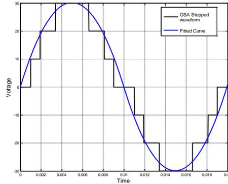
Fig. 5(b) Piecewise Curve fitted Voltage Waveform for GSA.
