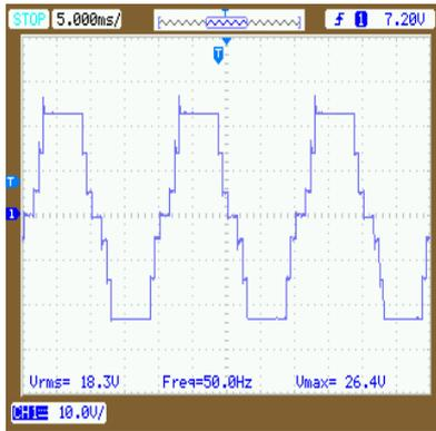
(a) Waveform obtained through PSO technique.
