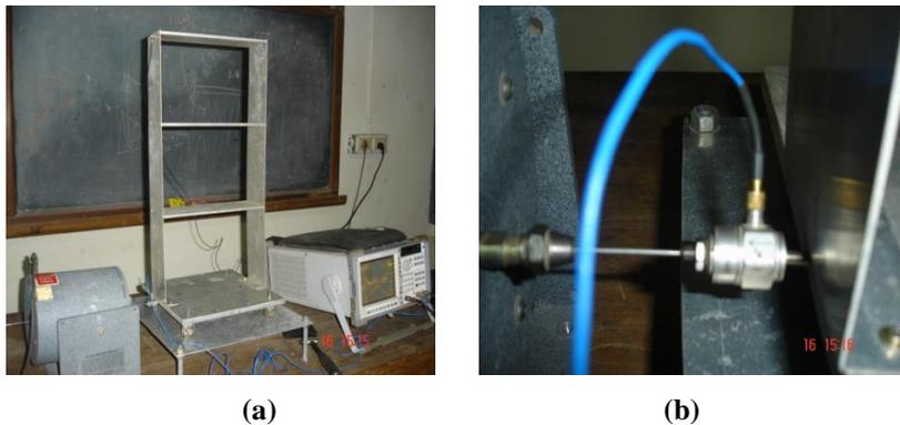
**Fig. 1. (a) Multilevel (three-level) structure for experiments, (b) Zoomed view of electro-dynamic shaker connected to base.**
