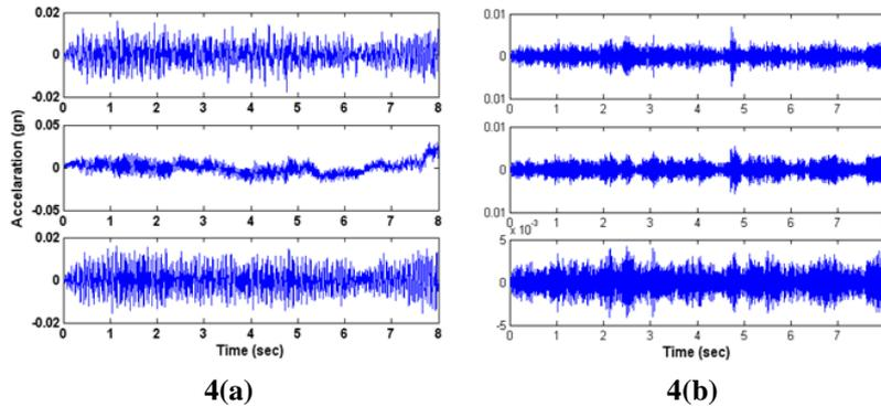
**Fig. 4. (a) Acceleration time history responses for level3 (top), level2 (middle), level1 (bottom) respectively (b) IMF1 for level3 (top), level2 (middle), level1 (bottom) for band limited white noise input (modification mass (50gm) placed on level 3 at approximately 4.7 s).**
