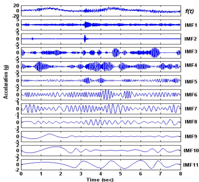
Fig. 3. The response signal and its intrinsic mode functions.
