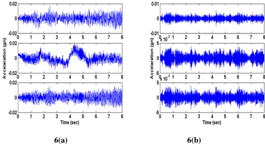
**Fig. 6. (a) Acceleration time history responses for level3 (top), level2 (middle), level1 (bottom) respectively (b) IMF1 for level3 (top), level2 (middle), level1 (bottom) for band limited white noise input (modification mass (50gm) placed on level 1 at approximately 4.3 s).**
