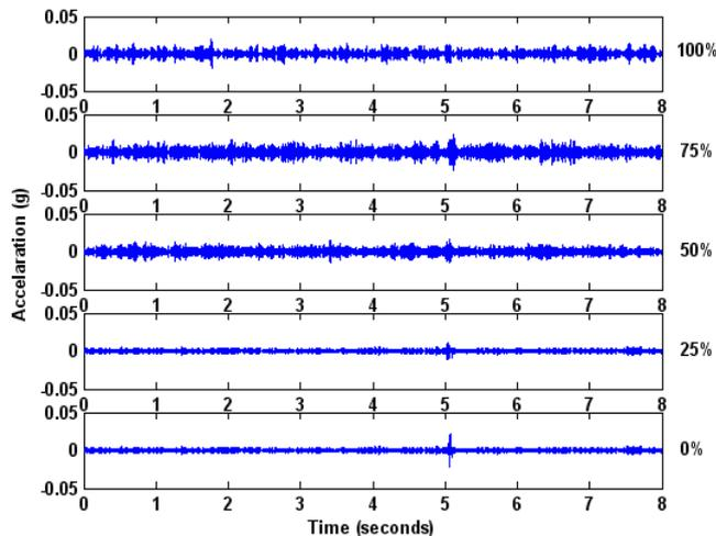
**Fig. 10. IMF1 for top level with modification of mass placed approximately at 5 s. noise added to input excitation (a) noise level 100% of original input RMS value (b) 75% (c) 50% (d) 25% (e) 0% (no noise).**
