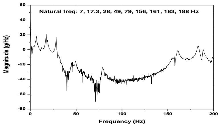
**Fig. 2. Natural frequencies lie between 0 to 200 Hz.**
