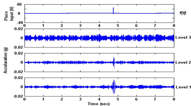
**Fig. 9. (a) PZT actuator voltage input time history (b) IMF2 for level3, level2 and level1 for band limited white noise input (PZT actuator energized at 4.8 s to give impulse of 25V).**
