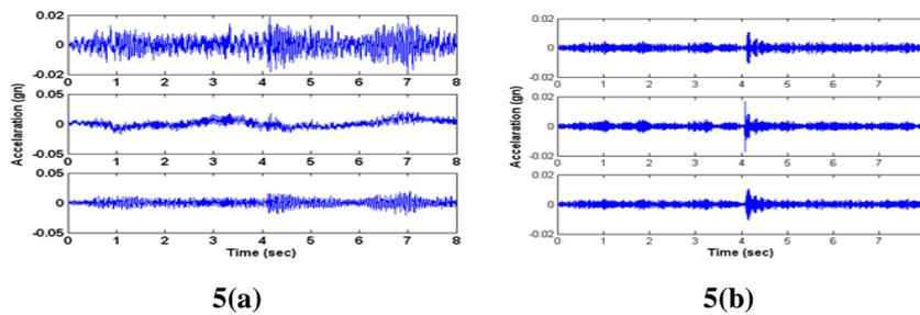
**Fig. 5. (a) Acceleration time history responses for level3 (top), level2 (middle), level1 (bottom) respectively (b) IMF1 for level3 (top), level2 (middle), level1 (bottom) for band limited white noise input (modification mass 50gm) placed on level 2 at approximately 4 s).**
