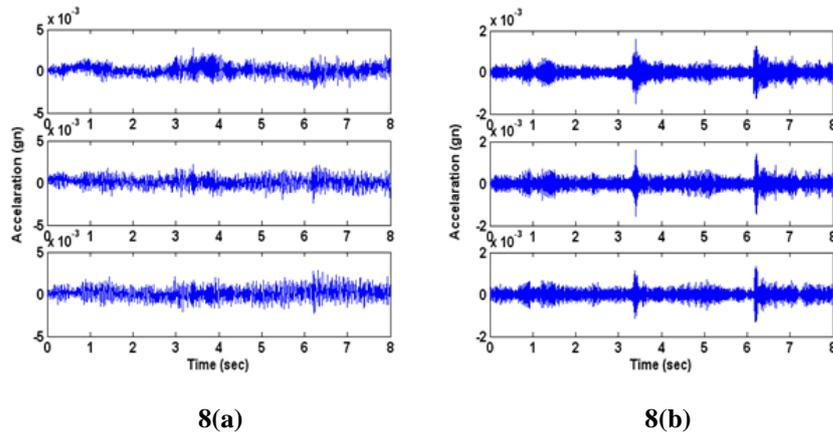
**Fig. 8. (a) Acceleration time history responses for level3 (top), level2 (middle), level1 (bottom) (b) IMF1 for level3 (top), level2 (middle), level1 (bottom) for band limited white noise input (modification mass (50 gm) placed on level 2 at approximately 3.2 and 6.2 s).**
