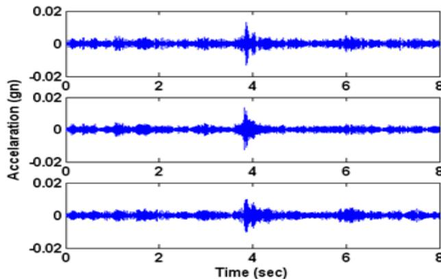
**Fig. 7. IMF1 for level3 (top), level2 (middle), level1 (bottom) for band limited white noise input (modification mass 100gm) placed on level 2 at approximately 4.s).**
