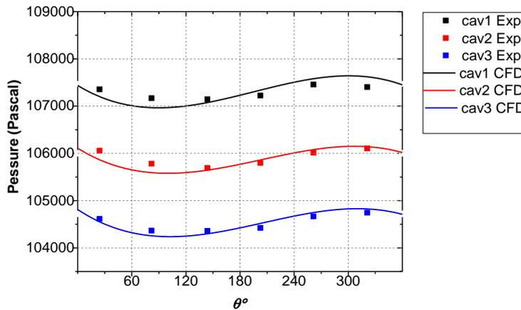
**Fig. 7. CFD and experimental pressure distribution in the circumferential direction at the mid-cavities of the seal.**
