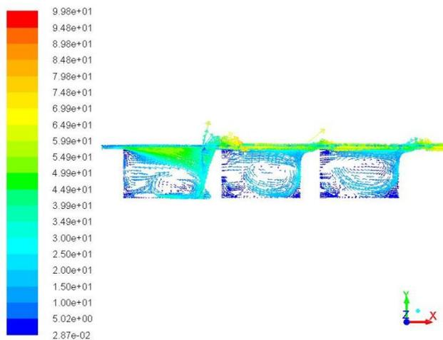
**Fig. 9. Velocity vectors in the XY plane of the seal.**
