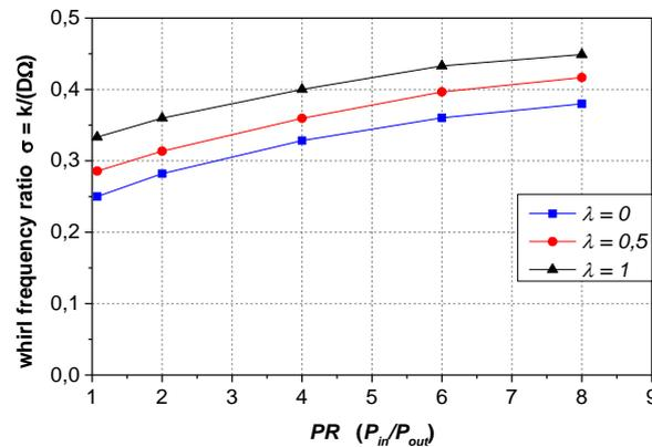
**Fig. 16. Whirl frequency ratio versus pressure ratio with the inlet swirl ratio as a parameter.**
