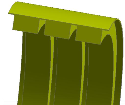
Fig. 2. A cut section of the 3-D computational domain of the seal.
