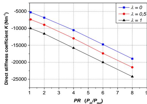
Fig. 12. Direct stiffness coefficient versus pressure ratio with the inlet swirl ratio as a parameter.
