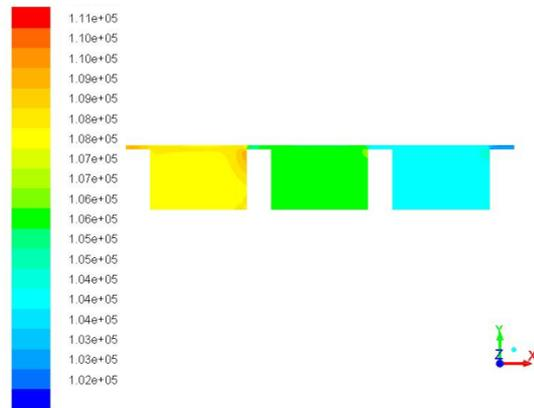
**Fig. 8. Pressure contours in the XY plane of the seal.**
