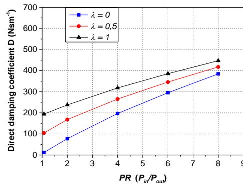
**Fig. 14. Direct damping coefficient versus pressure ratio with the inlet swirl ratio as a parameter.**
