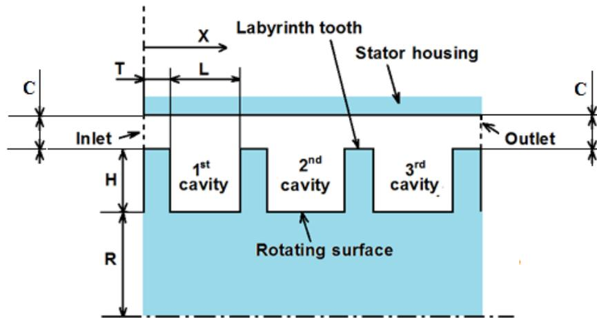
Fig. 1. Labyrinth seal geometry.
