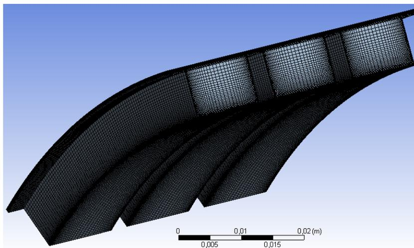
**Fig. 3. A cut section of the 3-D Mesh used for the fluid computational domain of the seal.**
