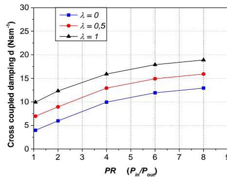
**Fig. 15. Cross damping coefficient versus pressure ratio with the inlet swirl ratio as a parameter.**
