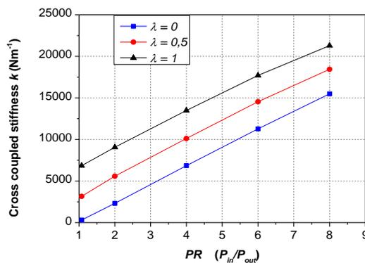
Fig. 13. Cross coupled stiffness coefficient versus pressure ratio with the inlet swirl ratio as a parameter.
