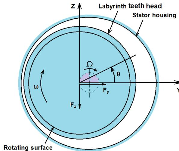
Fig. 5. Fluid forces induced in the seal.
