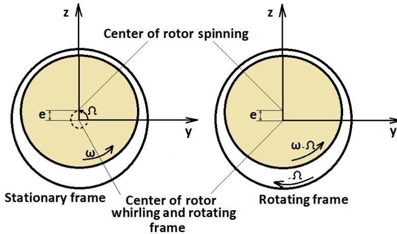
Fig. 4. Frame transfer from stationary to rotating.
