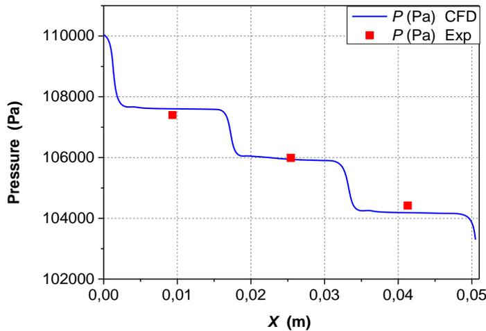
**Fig. 6. CFD and experimental pressure distribution in the axial direction of the seal.**
