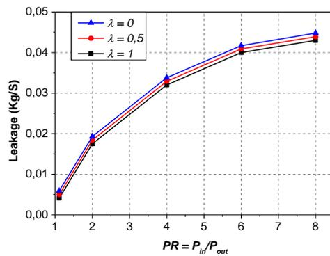
Fig. 10. Leakage flow versus pressure ratio with the inlet swirl ratio as a parameter.
