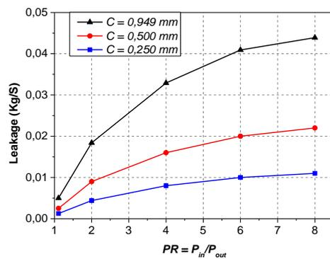
Fig. 11. Leakage flow versus pressure ratio with the mean radial clearance as a parameter.
