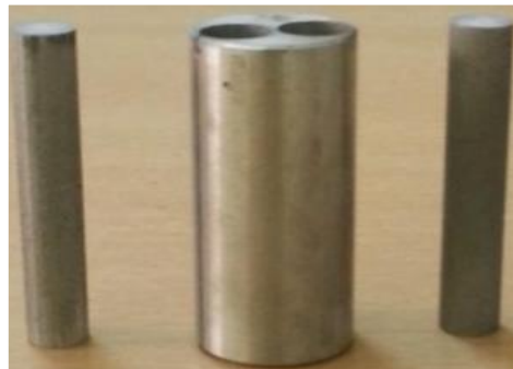
Fig. 2. Wear Specimen machined by EDM
