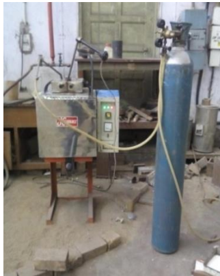
(a) Melting Furnace with Argon Gas arrangement
