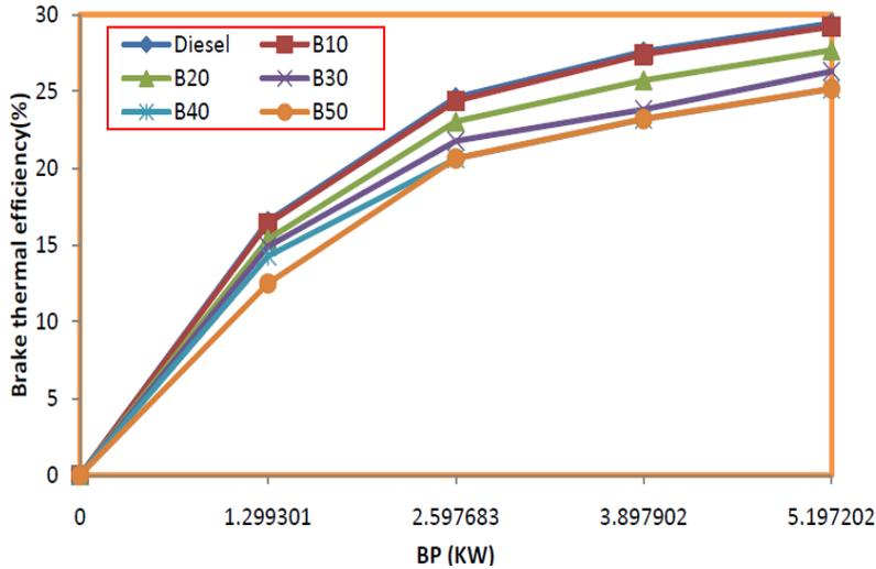
**Fig. 4. Brake thermal efficiency vs. BP for different blends.**
