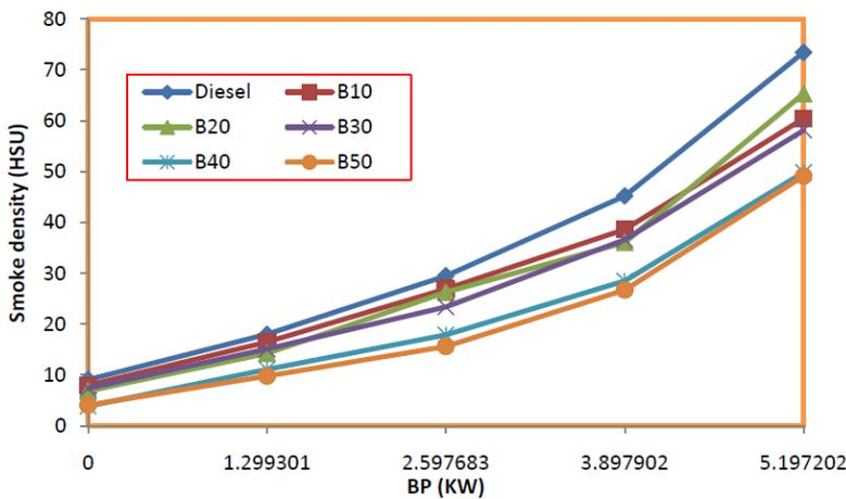
**Fig. 5. Smoke density vs. BP for different blends.**
