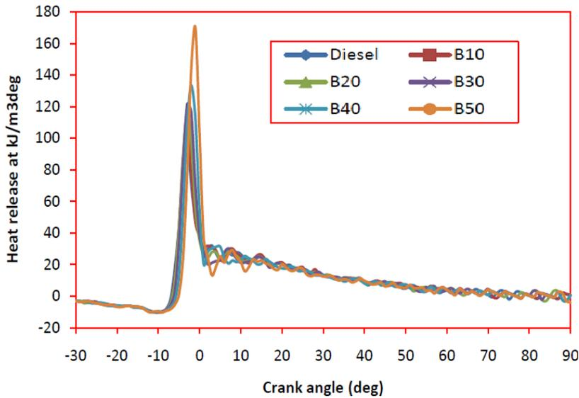
Fig. 8. Heat release rate vs. BP for different blends.
