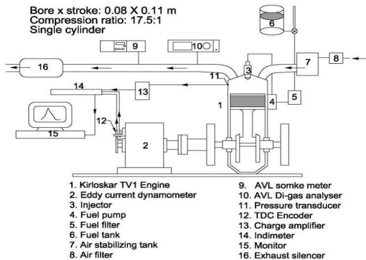
**Fig. 2. Experimental setup.**
