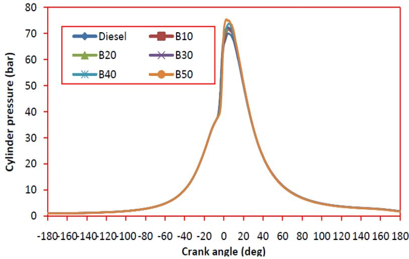
Fig. 7. Cylinder pressure vs. BP for different blends.
