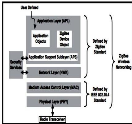
Fig. 5. ZigBee architecture.
