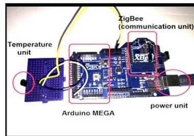
**Fig. A-4. Temperature end device.**
