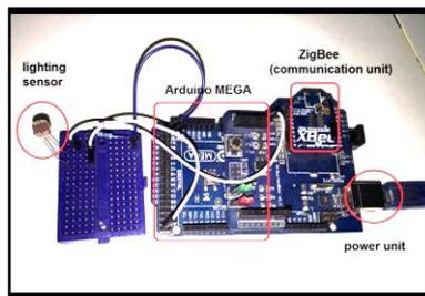
**Fig. A-3. Lighting end device.**
