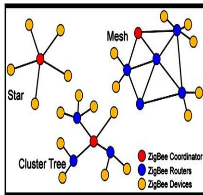
Fig. 6. The ZigBee topology.
