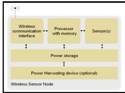
Fig. 3. Sensor node structure.
