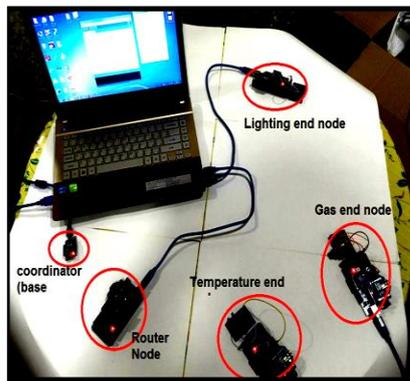
Fig. 8. Hardware design of full network.
