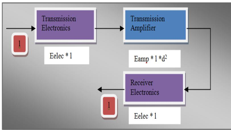
**Fig. 6. Transmission and reception energy model.**
