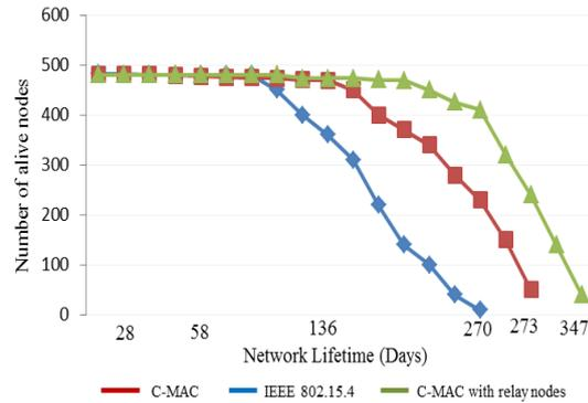
**Fig. 24. The effect of different protocols on the percentage of alive nodes of 482 nodes.**
