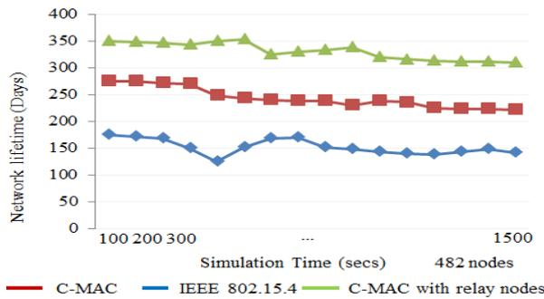
Fig. 13. The network lifetimes at different confidence intervals of 482 nodes.
