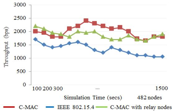
**Fig. 16.** The effect of C-MAC on the throughputs at different confidence intervals of 482 nodes.
