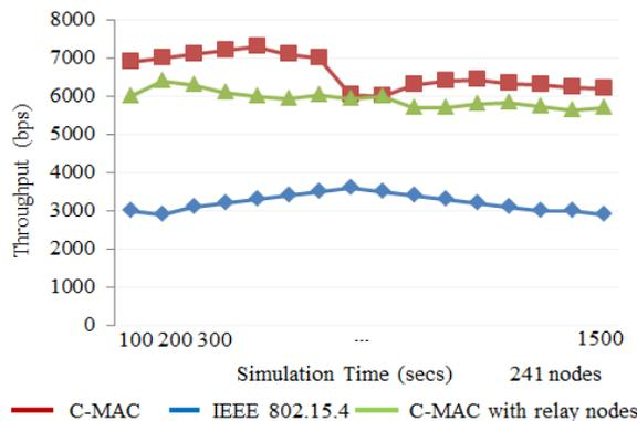
Fig. 15. The effect of C-MAC on the throughputs at different confidence intervals of 241 nodes.
