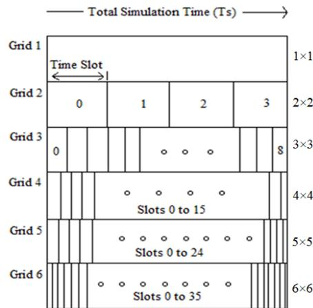
**Fig. 9. The number of time slots in different layers of concentric square grids  $G_i$ .**
