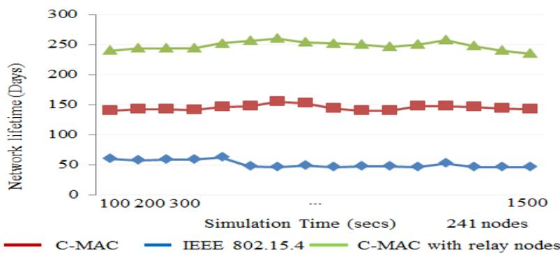
Fig. 12. The network lifetimes at different confidence intervals of 241 nodes.
