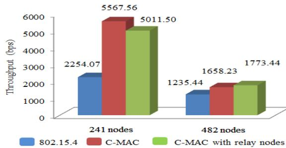
Fig. 14. The comparison of the throughputs of 241 and 482 nodes.
