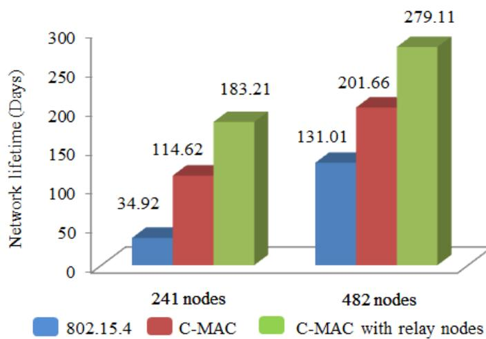
Fig. 11. The comparison of the network lifetimes of 241 and 482 nodes.
