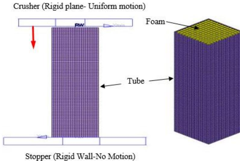
**Fig. 5. FE Modelling showing boundary conditions.**
