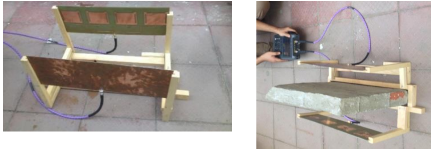
Fig. 21. Proposed measurement system using portable VNA.
