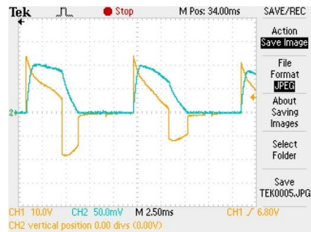
(a) without load-1550 rpm and V = 20V & I = 4.5A
