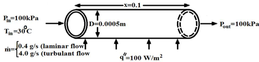
Fig. 1. Fluid flow through a circular micro channel.
