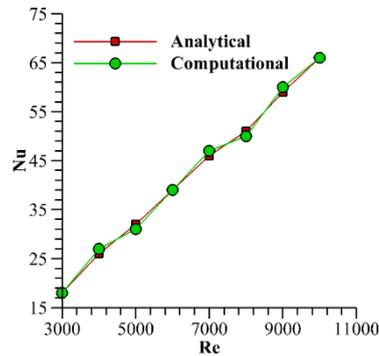
Fig. 5. Validation of Nusselt numbers of water at different Re.
