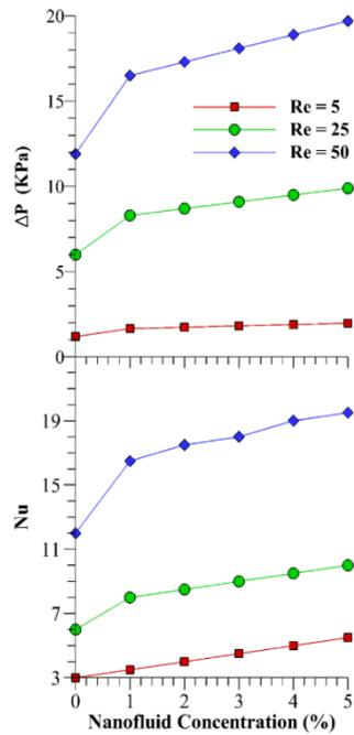
**Fig. 3. Nu and pressure drop at lower Re and nanofluid concentrations.**
